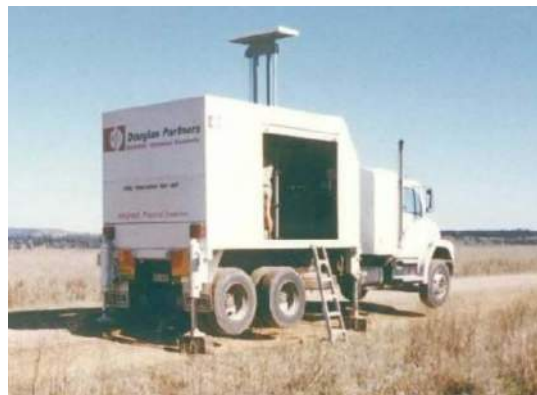
Figure 2: Purpose built CPT rig
