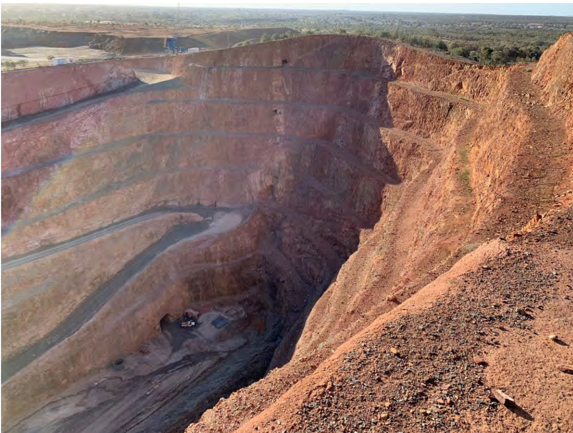
Plate 5.11 New Cobar Complex open cut showing the portal to underground workings (base of the pit)
