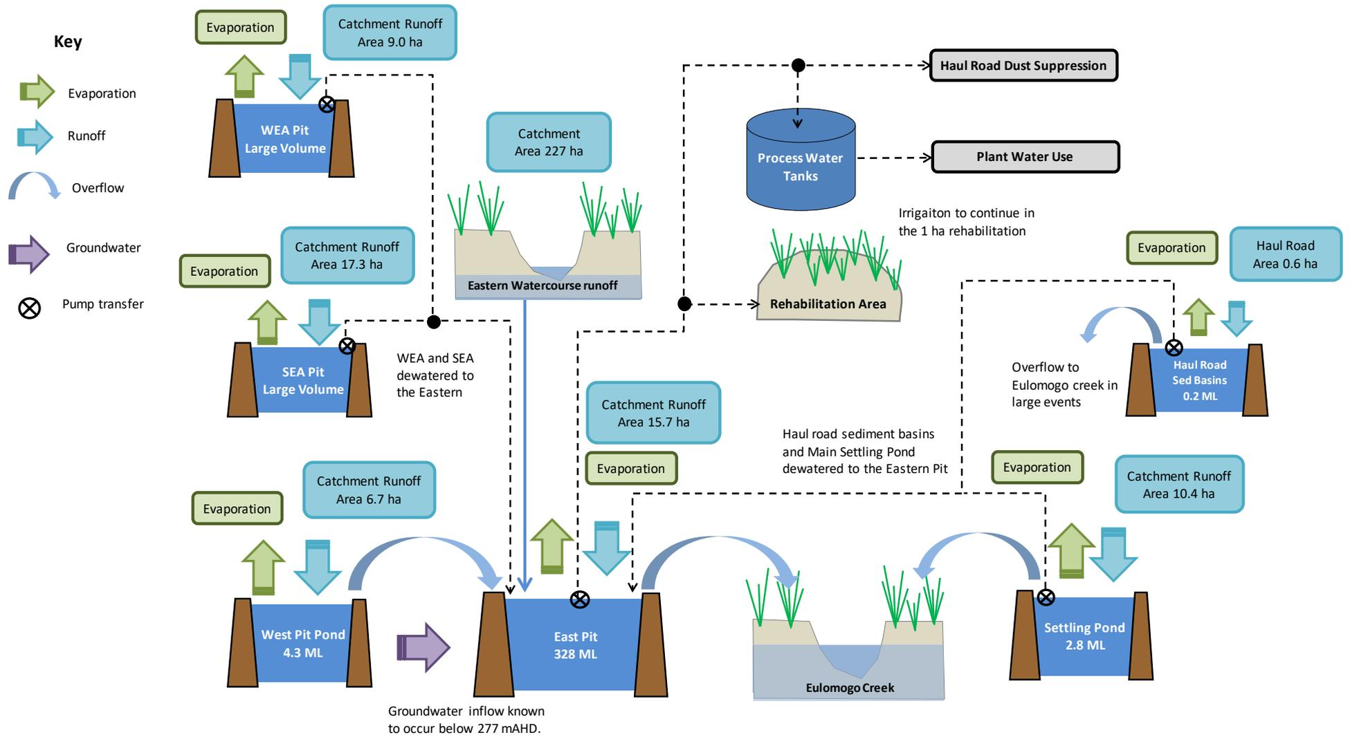
**Figure 5.1 Water management system functionality: proposed operations**
