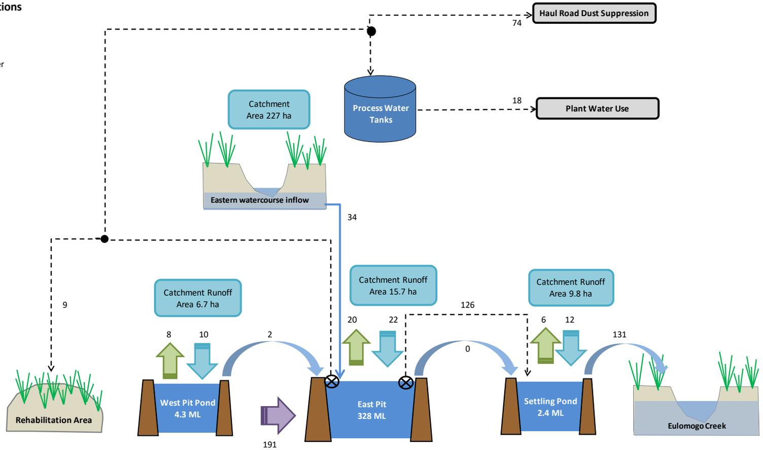
**Figure 4.3 Water balance: existing water management system – 10<sup>th</sup> percentile year**
