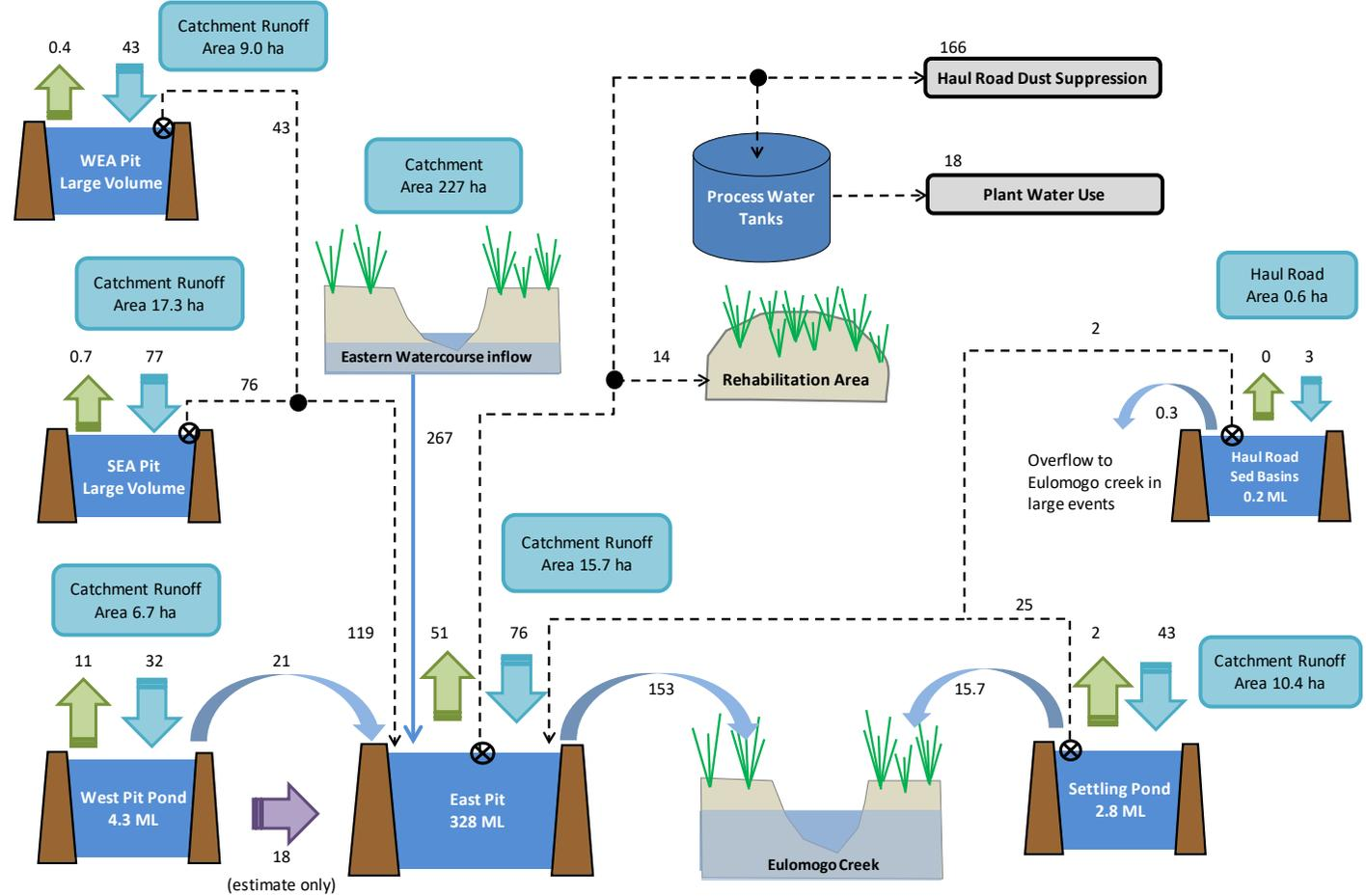
**Figure 5.5 Water balance: proposed operations – 90<sup>th</sup> percentile year**
