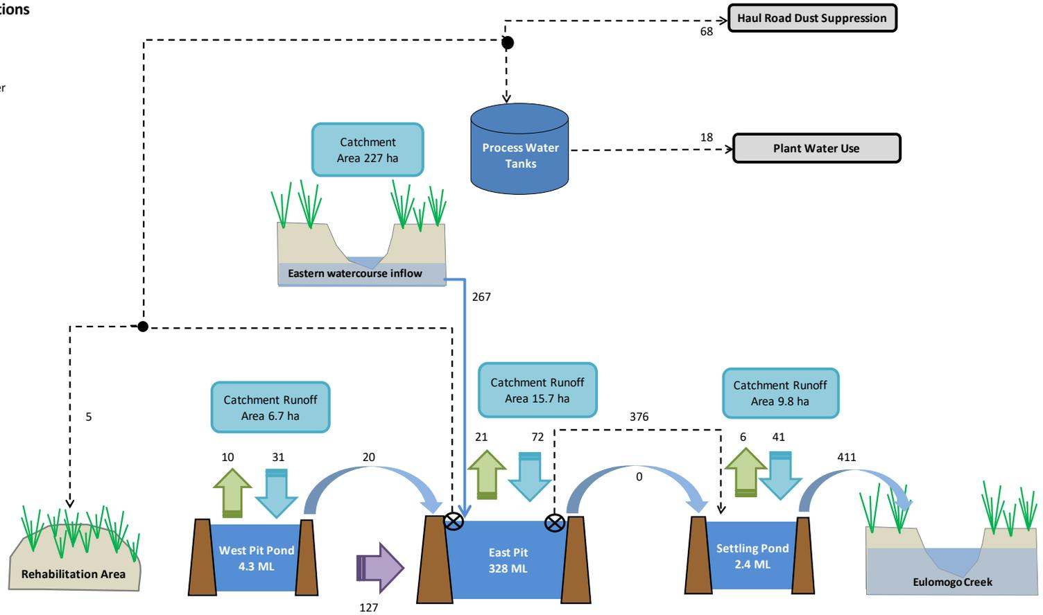
**Figure 4.5 Water balance: existing water management system – 90<sup>th</sup> percentile year**
