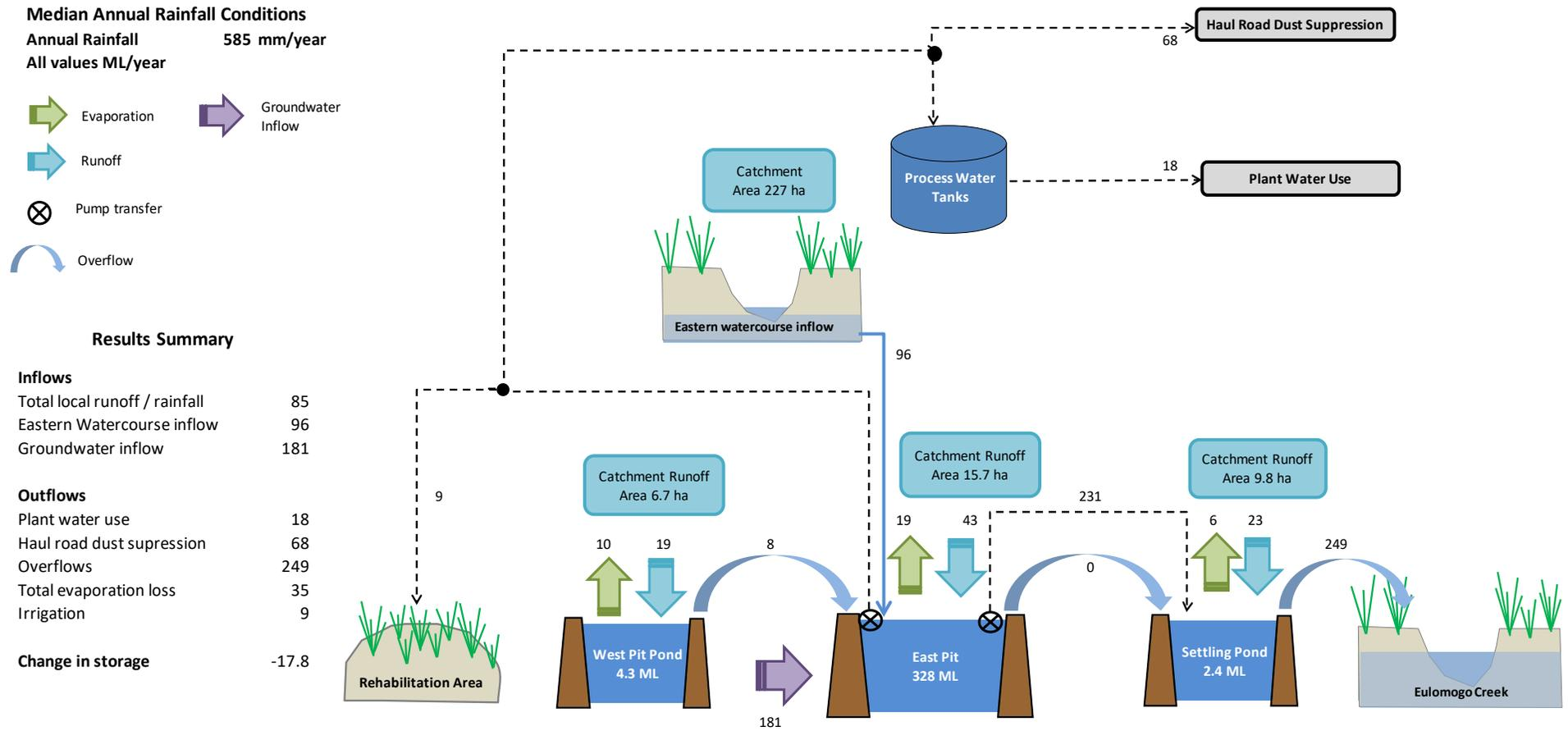
**Figure 4.4** Water balance: existing water management system – 50<sup>th</sup> percentile year
