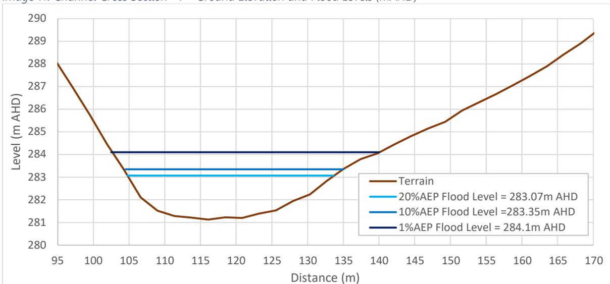
Image 12: Channel Cross Section #2 – Ground Elevation and Flood Levels (mAHD)
