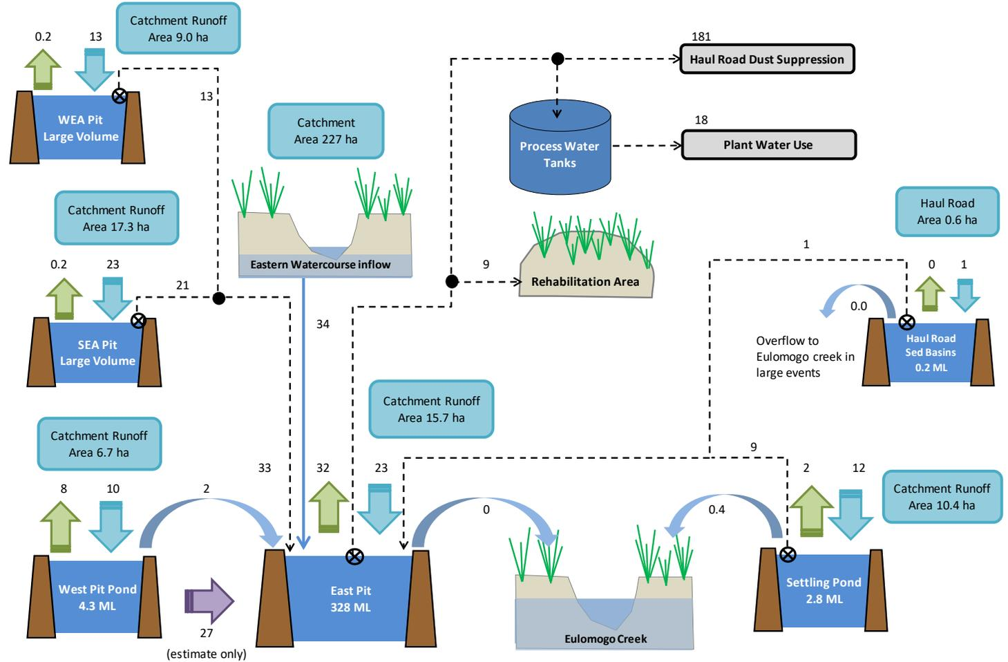
**Figure 5.3 Water balance: proposed operations – 10<sup>th</sup> percentile year**
