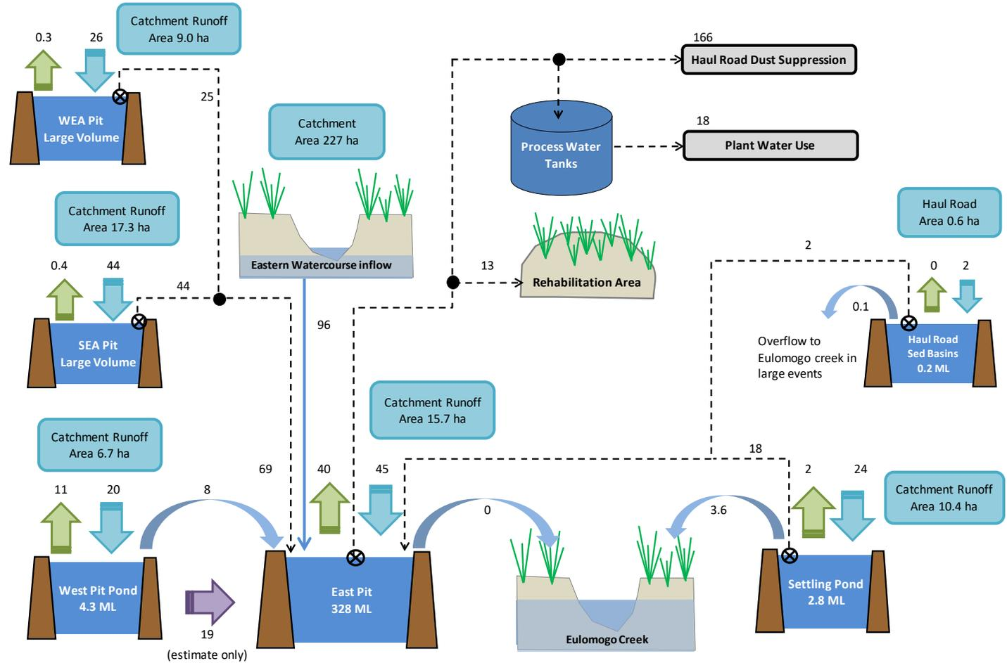
**Figure 5.4 Water balance: proposed operations – 50<sup>th</sup> percentile year**
