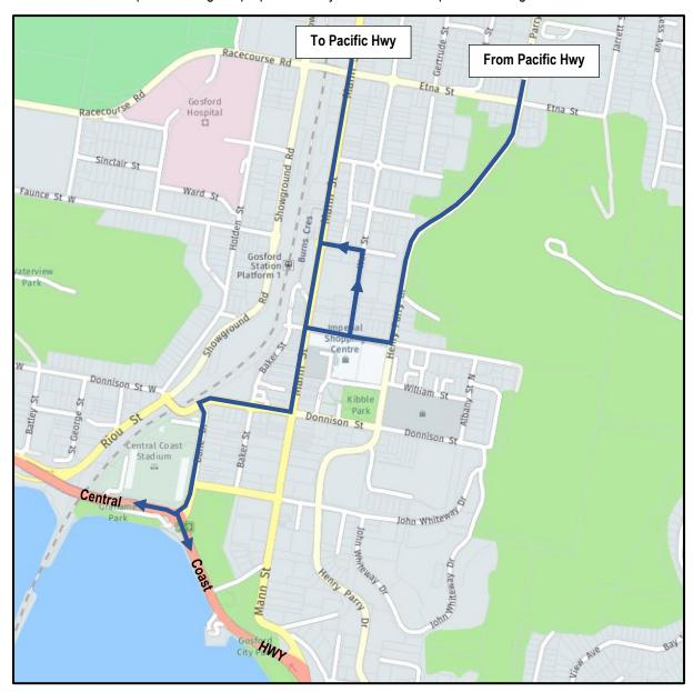
Figure 5-1 - Vehicle movement plan (two-way) for heavy construction traffic
