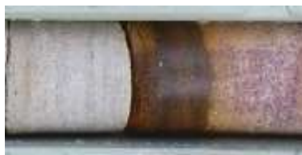
Photograph 5: Bedding conformable ironstone band in sandstone. DMDDH09, 41.4 to 41.55m. This is typical of most of the ironstone occurring on the site.
