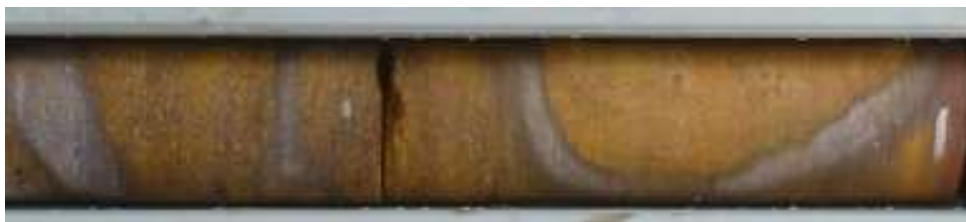
Photograph 6: Liesegang banded ironstone developed in sandstone. DMDDH09, 28.4 to 28.8m. Less often occurring form of ironstone, but often quite thick where it does occur.
