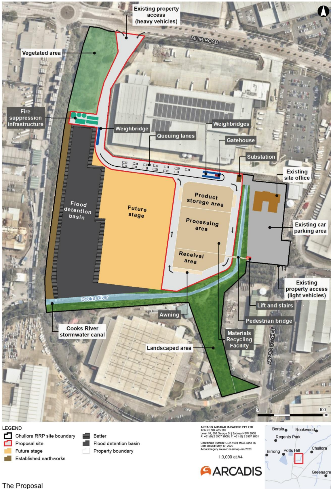
Figure 2 Proposed MRF layout (provided by Arcadis)
