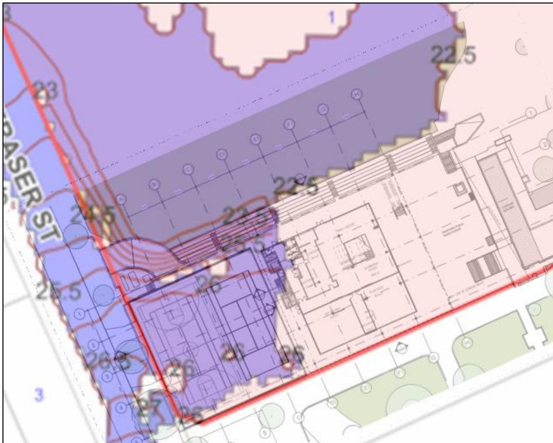
**Figure 3 – 1% AEP Flood Extent and Elevation as Identified by Council via email correspondence, overlaid on proposed layout (29.01.2020)**
