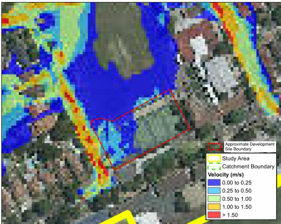
1% AEP Flood Velocity (extracted from Figure 18Fii in the Powells Creek and Salesyards Creek Revised Flood Study (2016))
