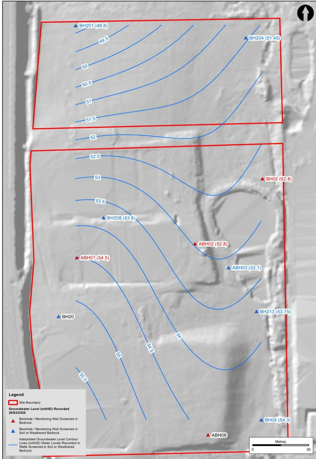
Figure 6: Groundwater levels recorded 28 February 2020 and interpreted groundwater flow direction.
