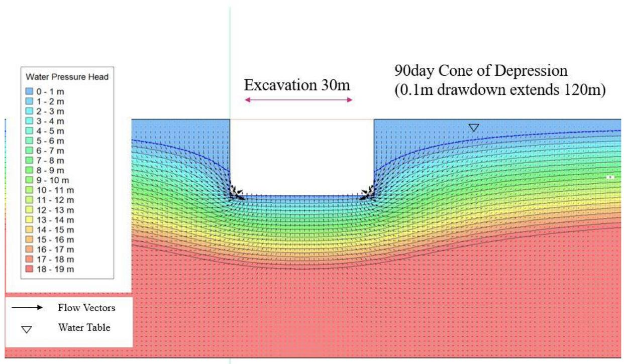
Figure 10: 2D numerical simulation output (SEEPW software) of potential groundwater ingress into the waste bunker excavation.
