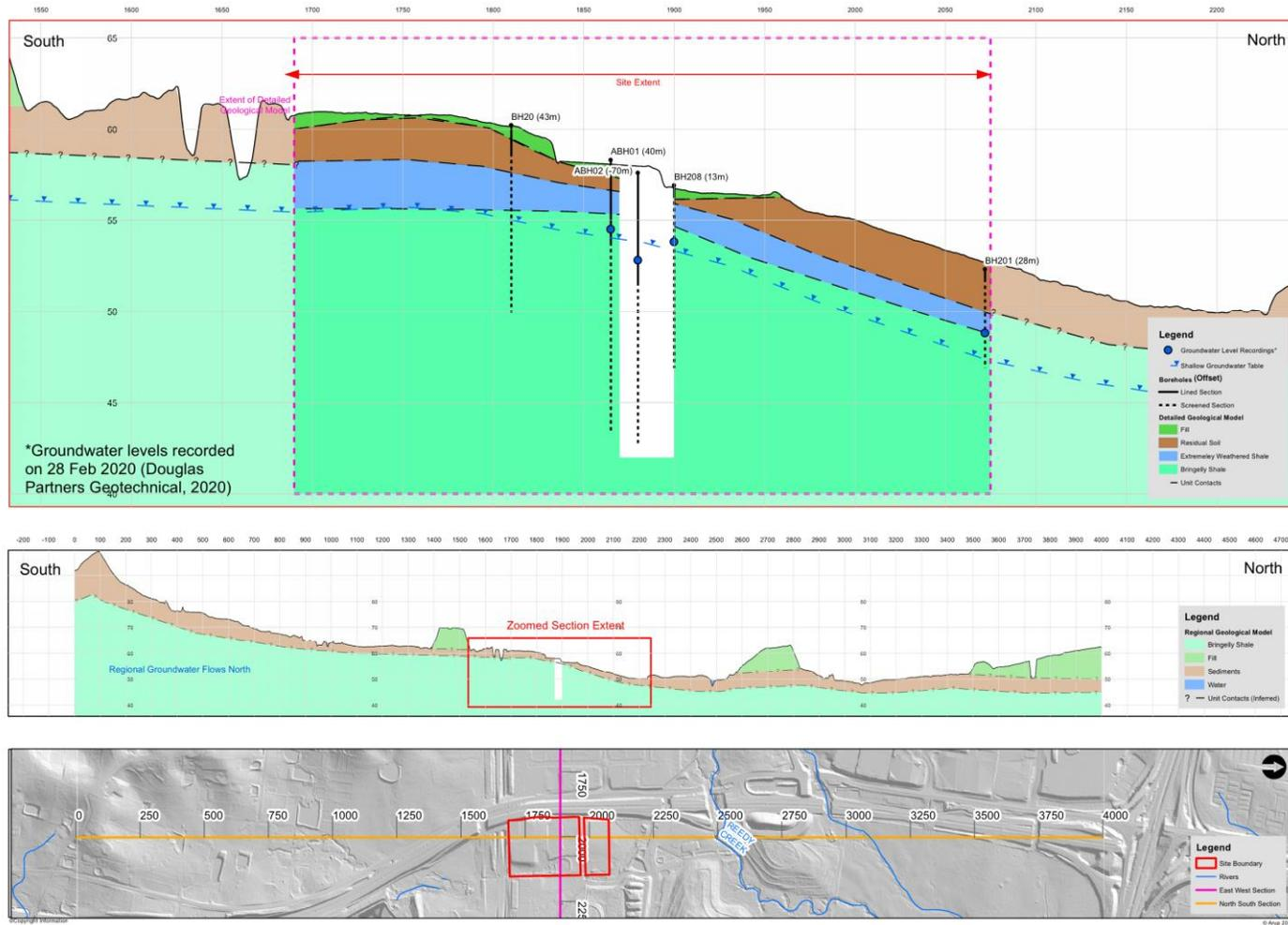
Figure 8b: North-south soil and water conceptual cross-section of site
