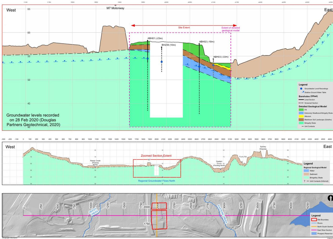
Figure 7a: East-west soil and water conceptual model cross-section of site
