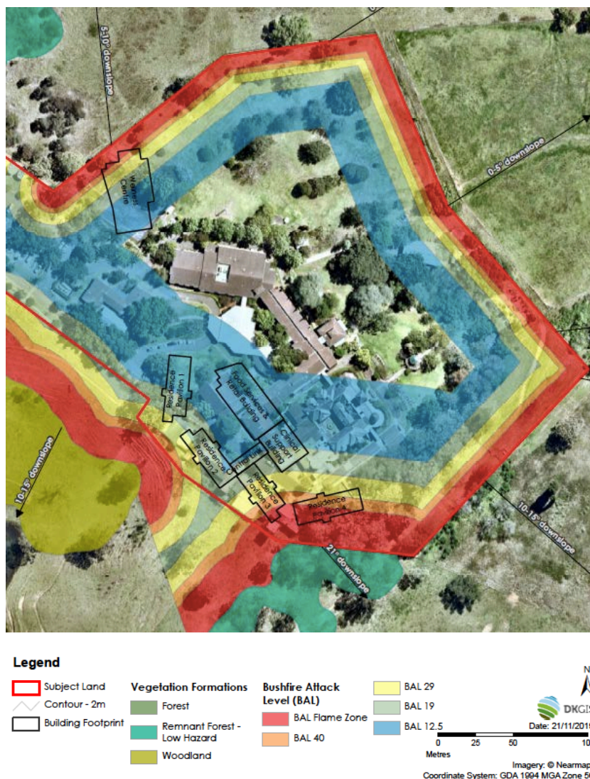
Figure 47. Bushfire attack levels – option 2 (without easement) Source: Blackash
