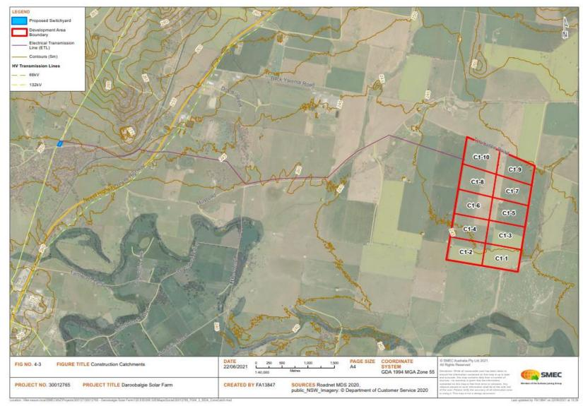
Figure 4-3 Proposed construction catchments at the solar farm site
