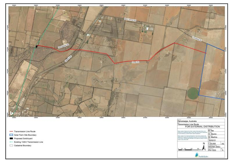
Figure 4-1 Transmission line route (shown in red), the switchyard site (shown in black) and part of the solar farm site (shown in blue)
