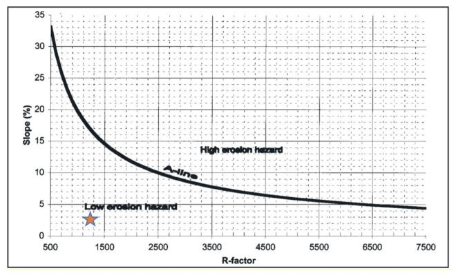
Figure 4-2 Assessment of potential erosion hazard
