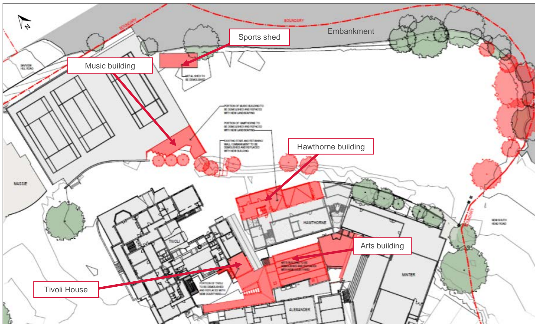
Figure 25 | Demolition plan (Source: Applicant's EIS 2020)
