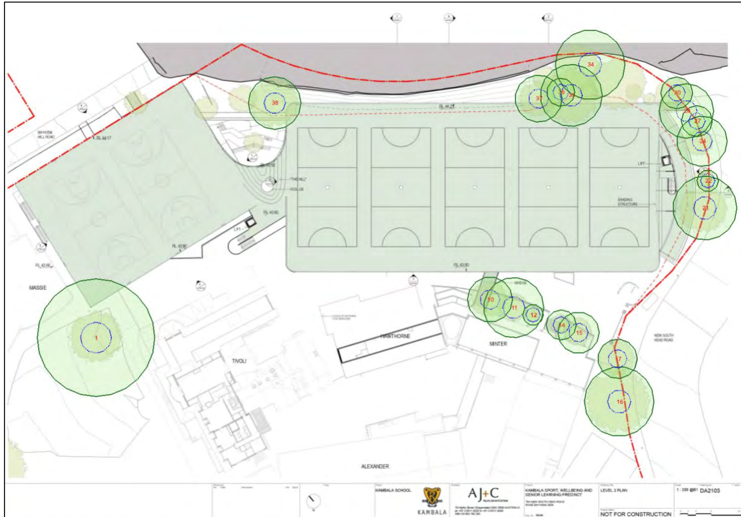
PLAN OF SITE SHOWING TREES TO BE PROTECTED (TPZ OUTER GREEN CIRCLE, SRZ DASHED INNER CIRCLE) - TPZ FENCING INSTRUCTIONS IN SECTION 11.1.
