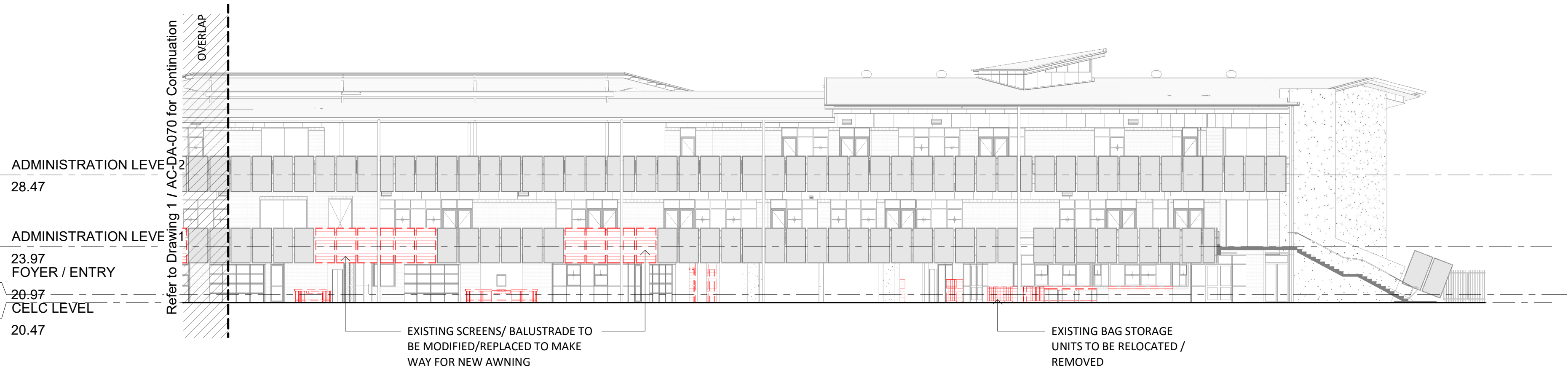
2 EAST ELEVATION - DEMOLITION - PART 2 1 : 200
