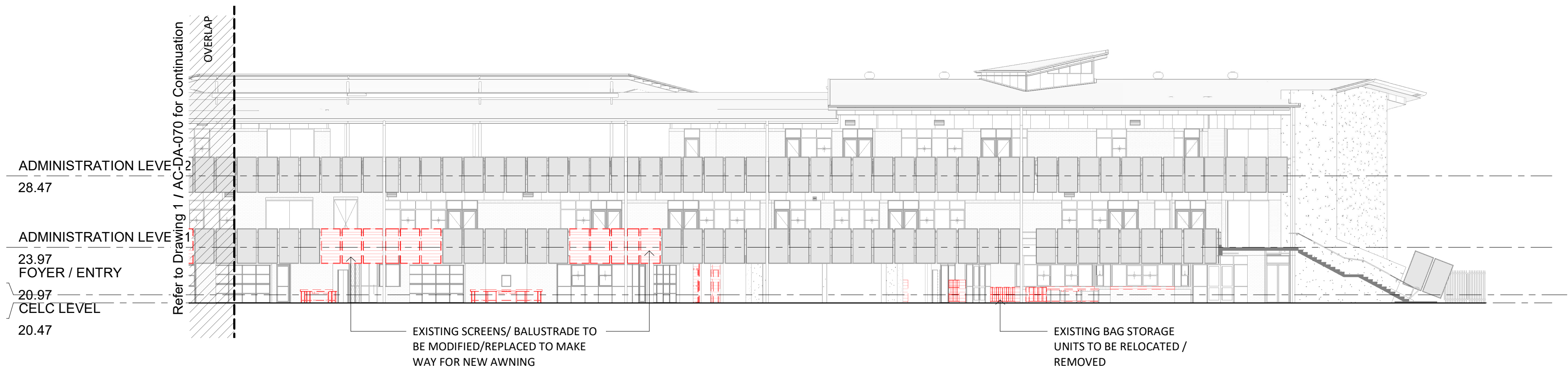
2 EAST ELEVATION - DEMOLITION - PART 2 1 : 200
