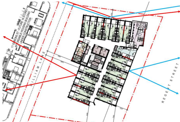
Figure 26 Possible Reflection Conditions Upper Levels
