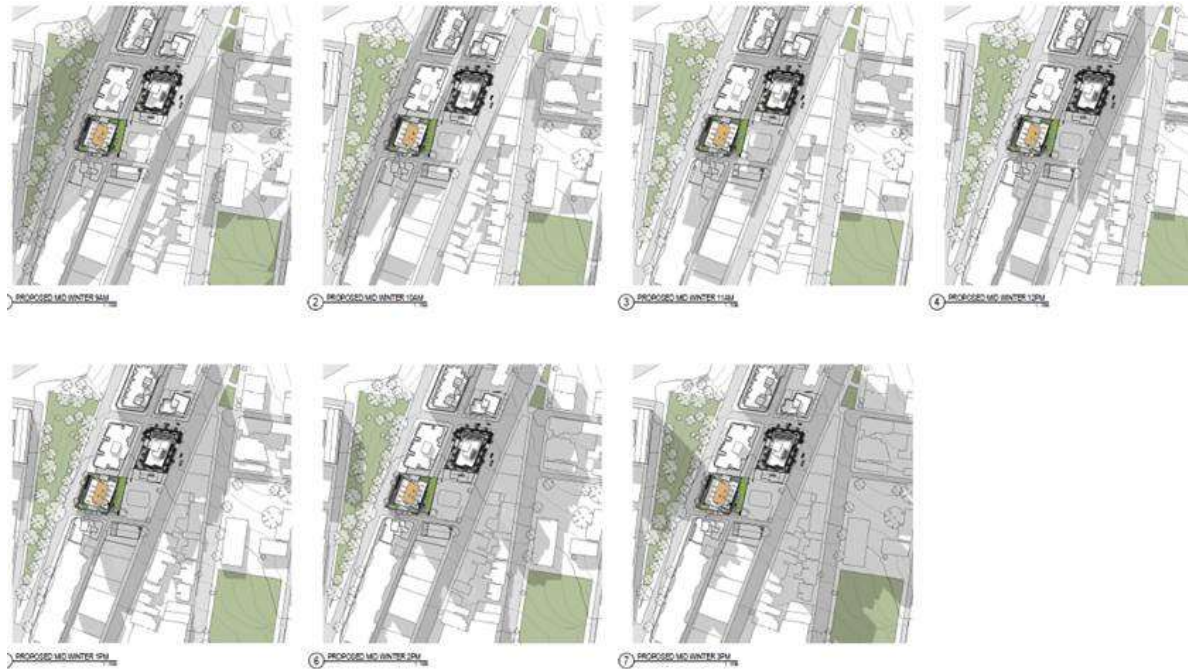
Figure 23 Solar Analysis of proposed built form during winter solstice
