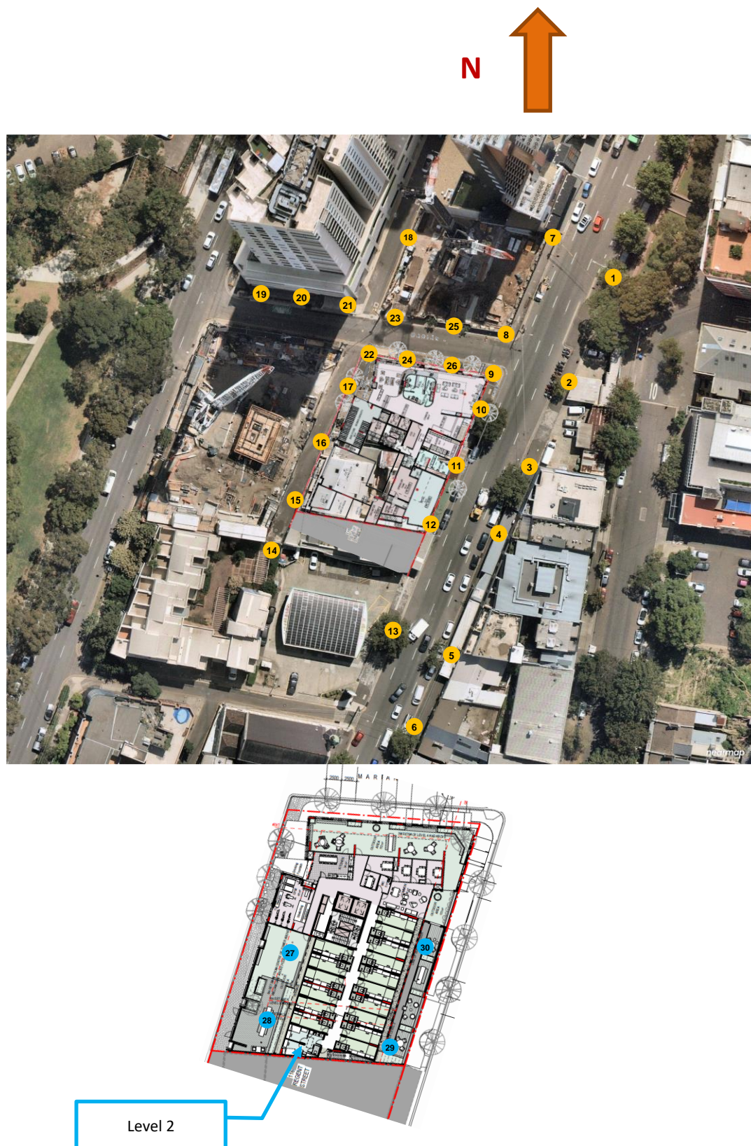
Figure 9 Wind Tunnel Test Sensor Locations
