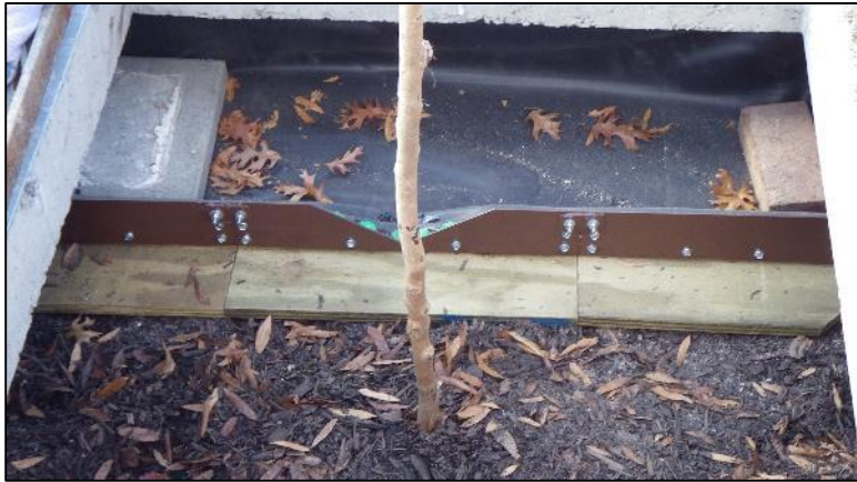
Figure 22. Inflow compound weir for flow measurement
