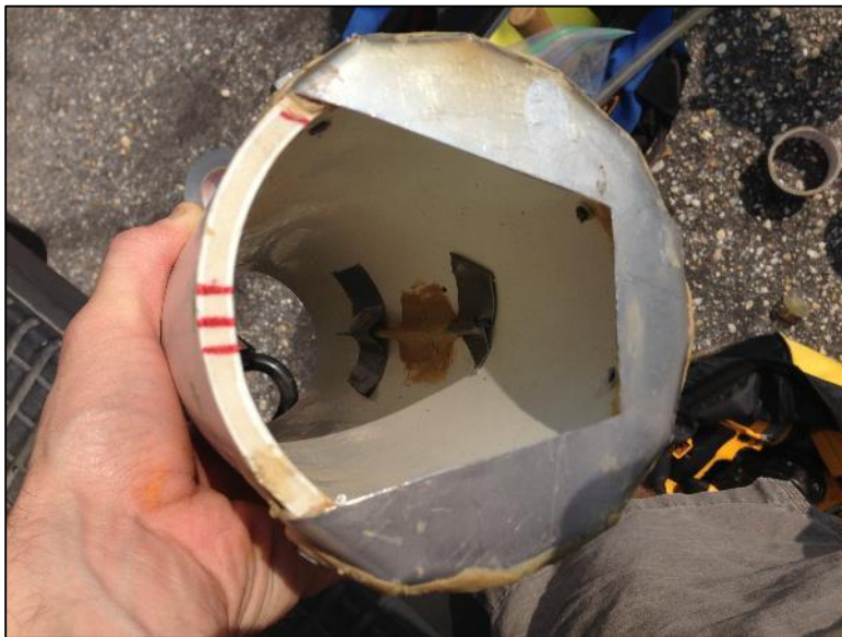
Figure 23. Primary measuring device on the outlet pipe (Cipolletti-style weir)
