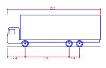
HRV - Heavy Rigid Vehicle Overall Length Overall Width Overall Body Height Min Body Ground Clearance Track Width Lock-to-lock time Curb to Curb Turning Radius
