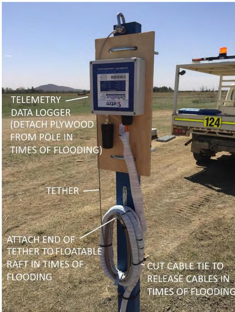
Figure 7: Telemetry installation
