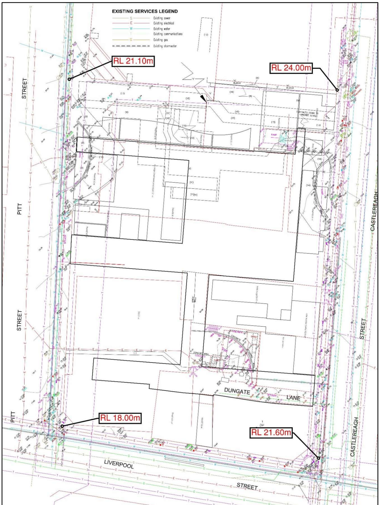
Figure 3: Existing Services and Site Levels Approximate)
