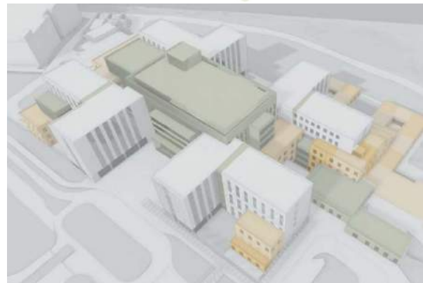
■ GRANULAR FORMS (PRE-CAST CONCRETE MASONRY) ■ RECESSIVE FORMS (WINDOW WALL)
