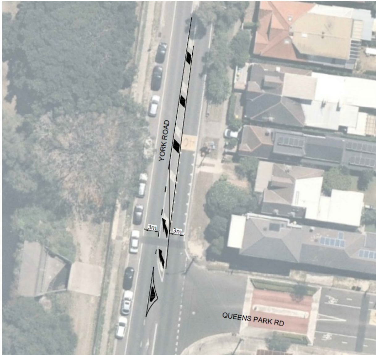
Figure 7.5: Concept Seagull Intersection Treatment
