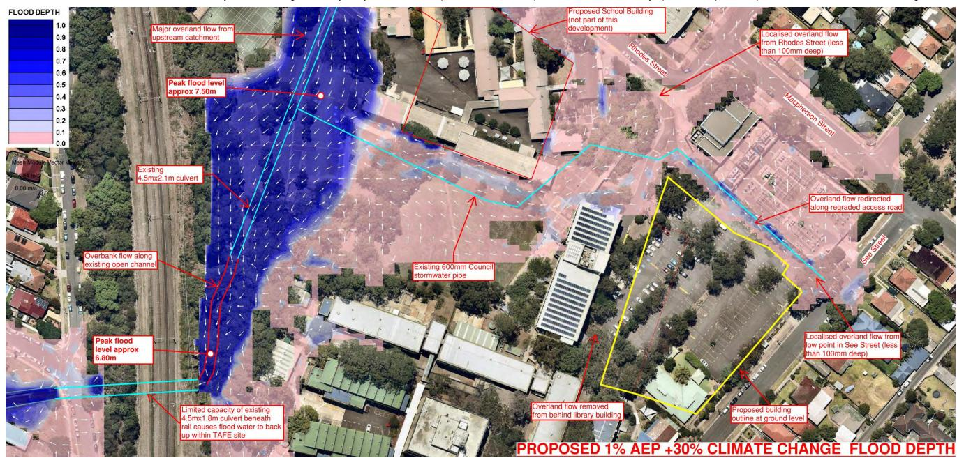
Figure 6.8.1 1% AEP Proposed Peak Flood Depths including 30% Climate Change Impact
