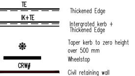
Wall detailed by structural engineer notcrete Wall detailed by DEJ Dowelled expansion joint
