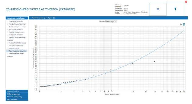
A separate RFFE model was obtained for the Commissioners Waters coinciding with the approximate location of the above gauge and the results estimate a 5% AEP flow of  $581m^3$ /s and a 1% AEP flow of 1,190m<sup>3</sup>/s. The 1% AEP flow closely matching that predicted by the RAFTS Model.
