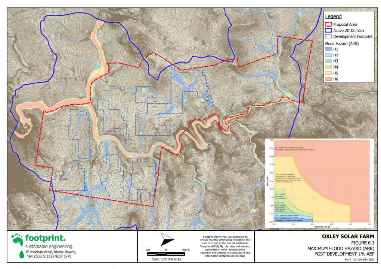
Figure 7-18 Post development 1% AEP hazard vulnerability (Footprint, 2021).
