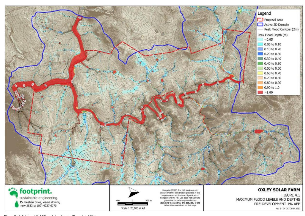
Figure 7-13 Existing 1% AEP peak flood levels (Footprint, 2021)
