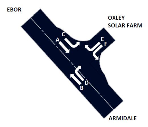
Figure 8-11 Traffic directions at Waterfall Way (Grafton Road) at Oxley Solar Farm site access.
