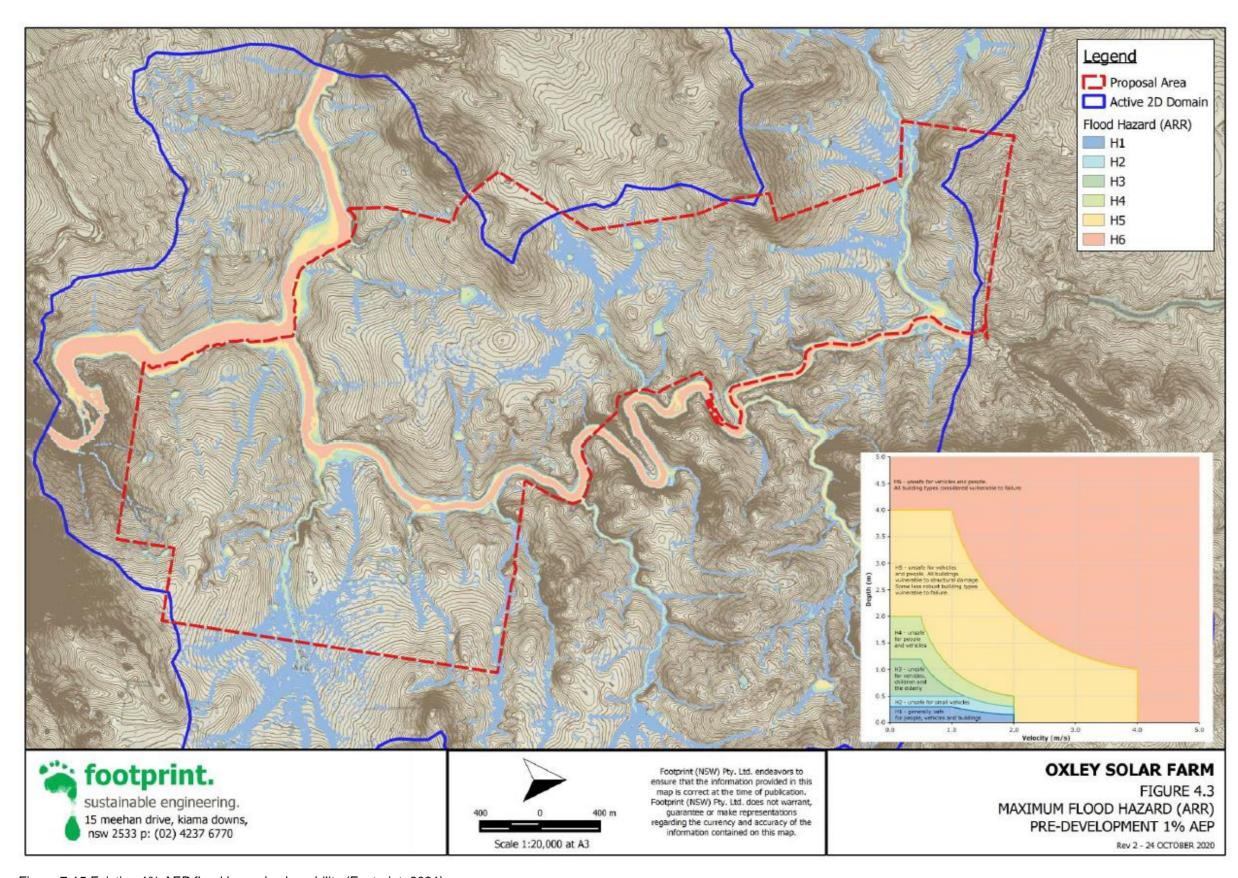
Figure 7-15 Existing 1% AEP flood hazard vulnerability (Footprint, 2021).
