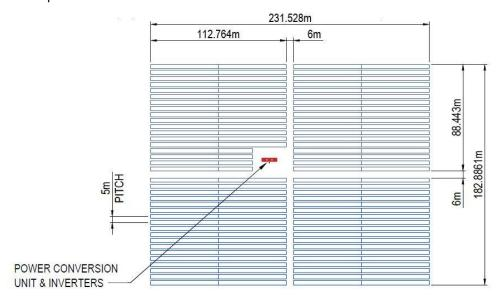
Figure 4-4 Typical array block showing location of PCU.
