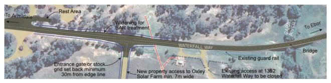
Figure 4-11 Concept Diagram of new property access arrangement to Waterfall Way (Grafton Road) (New England Surveying & Engineering, 2020).
