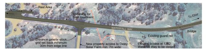
Figure 8-13 Concept Diagram of New Property Access Arrangement to Waterfall Way (Grafton Road).
