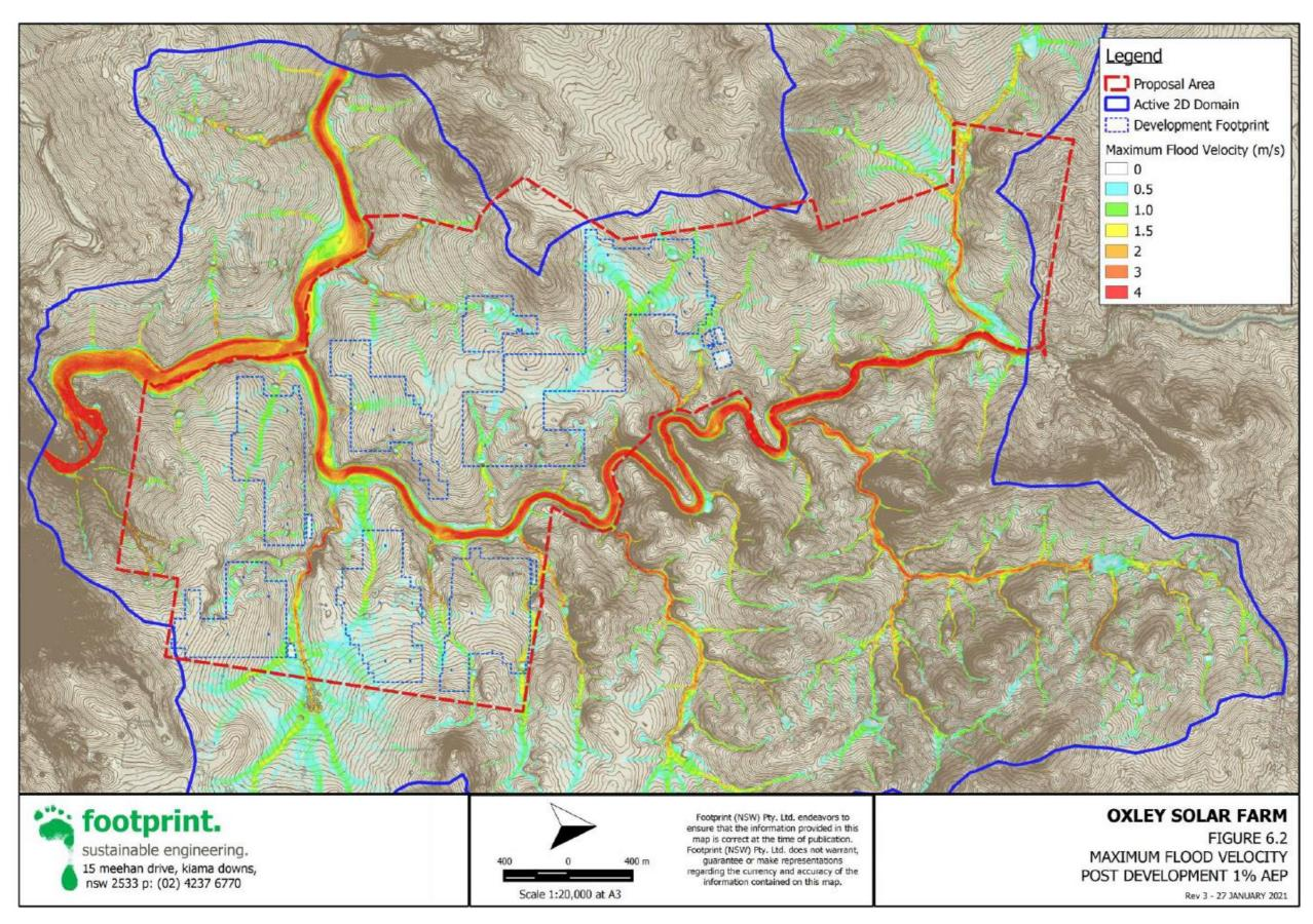
Figure 7-17 Post development 1% AEP peak flood velocities (Footprint, 2021).
