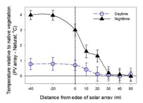
Figure 8-19 Measures of air temperature within and outside of the PV array (Barron-Gafford, 2018)
