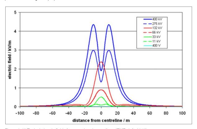
Figure 8-17 Typical electric fields from overhead powerlines (EMFs.info 2017).
