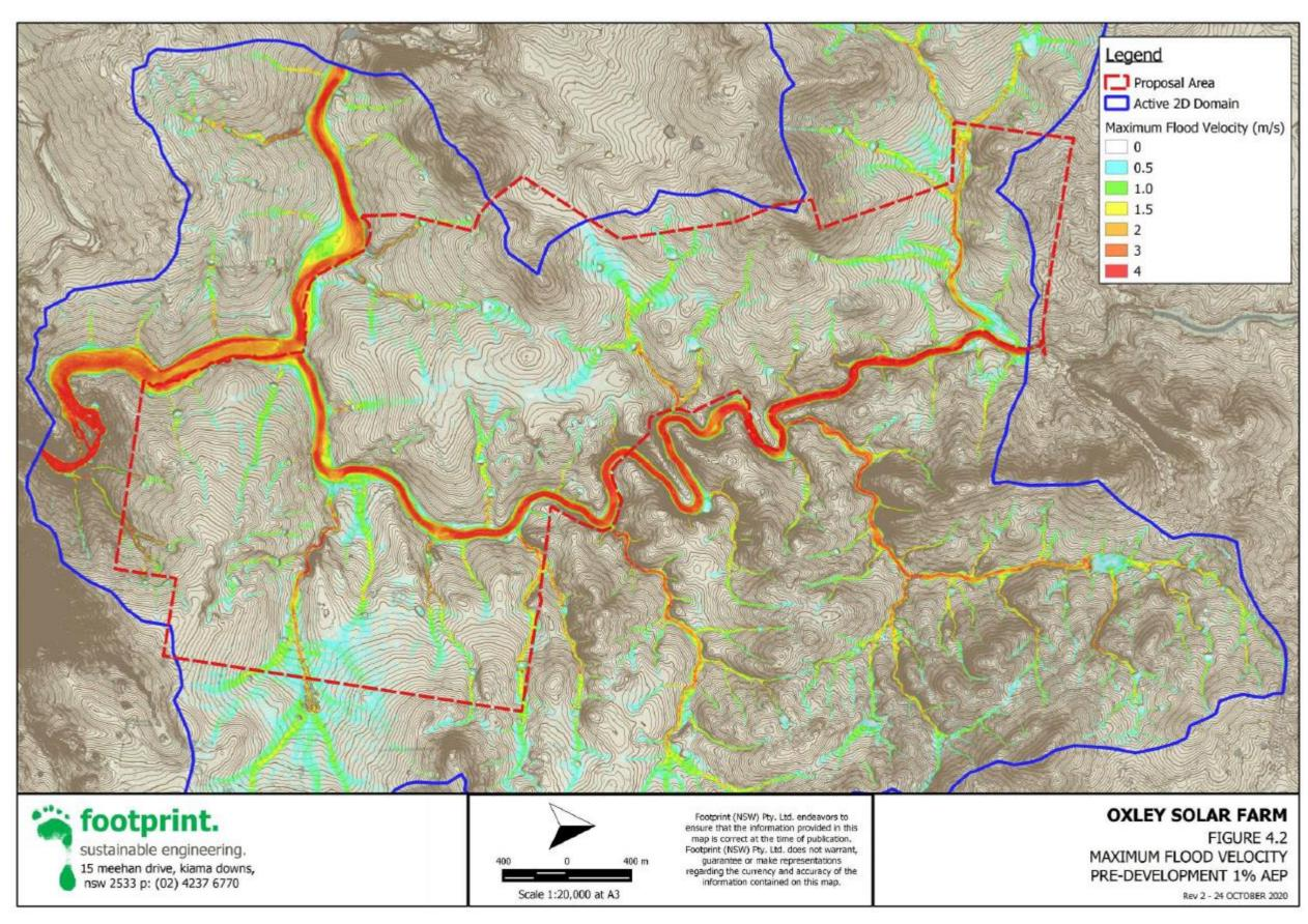
Figure 7-14 Existing 1% AEP Peak flood velocities (Footprint, 2021).
