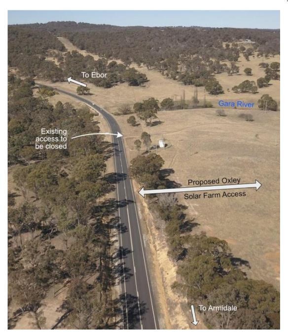
Figure 4-10 Proposed location for new property access to Waterfall Way (Grafton Road) (New England Surveying & Engineering, 2020).
