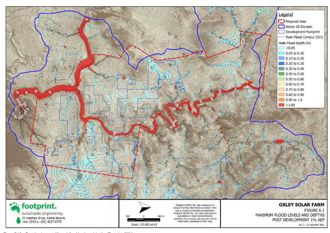
Figure 7-16 - Post development 1% peak flood levels and depths (Footprint, 2021).
