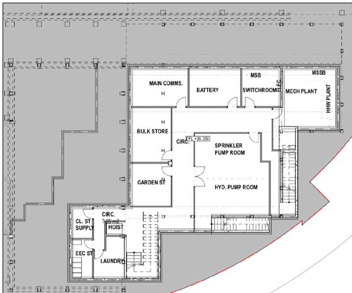
Figure 8.46: Proposed Lower Ground Layout, plant and facilities proposed for Building G basement (Source: FJMT, DA-2001, 18.12.19)
