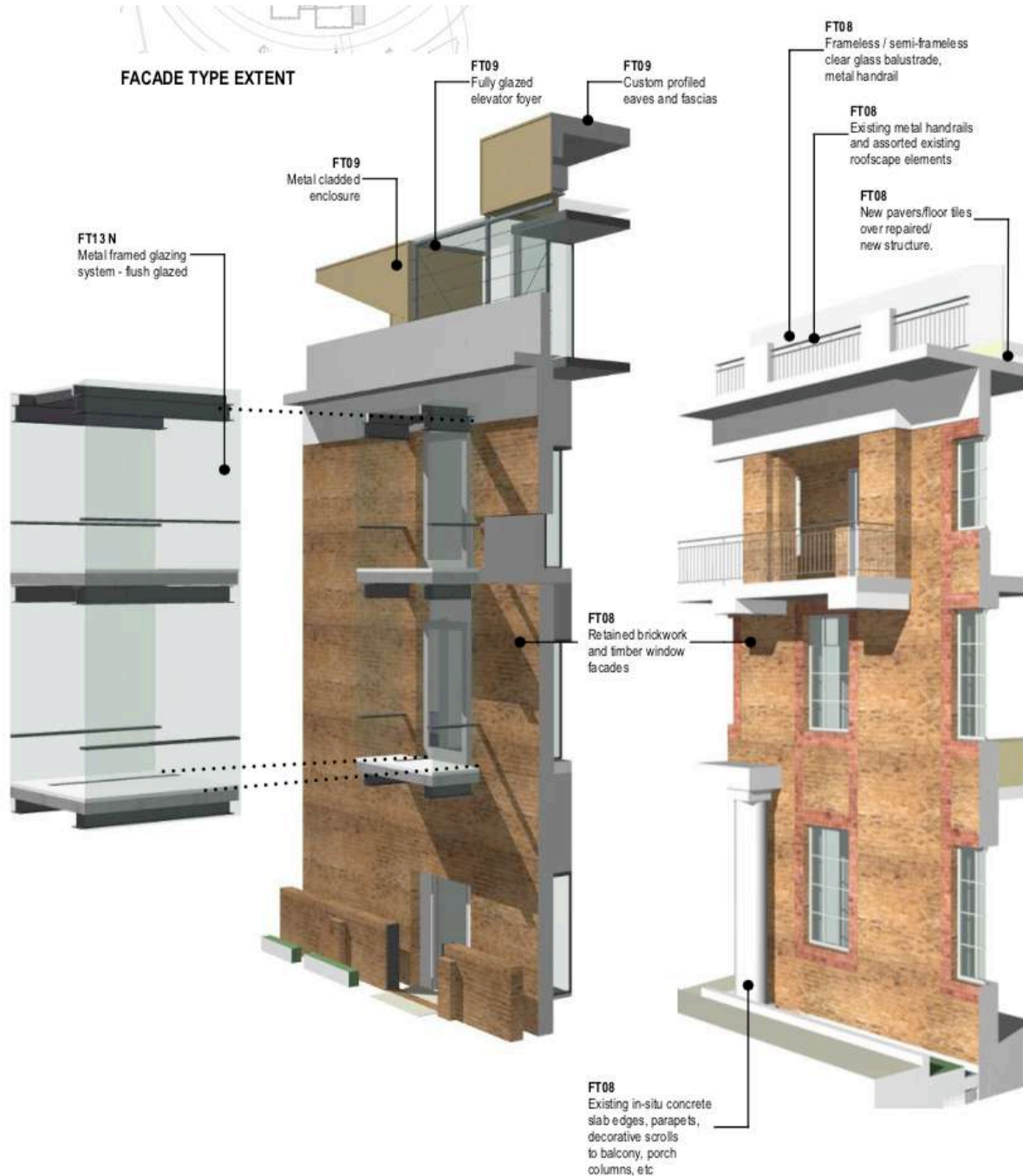
Figure 8.25: Building M Façade Type Extent – Retained brickwork and timber window facades, new elevator overrun/foyer and new Bridge Connection to MET (Source: FJMT 2020 SSDA Design Report: 65)
