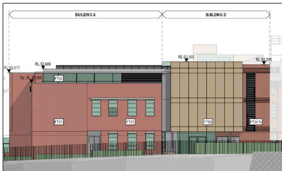
Figure 8.20: Setback of new storey addition from northern façade-northern elevation, allowing readability of original form of 1940s building. View from north (Source: FJMT DA-3001, SSDA01, 18.12.19)
