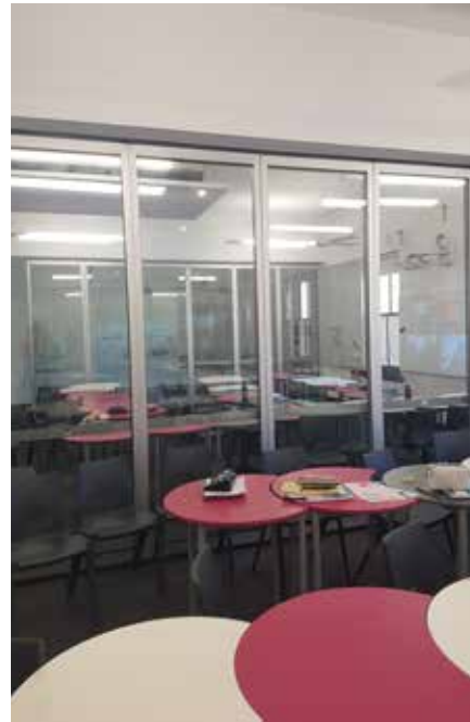
Figure 2.61: Level 3 classroom showing modern furniture, projectors and lowered false ceilings to accommodate services above. This former large space is now divided into three, by modern aluminium sliding door panels.
