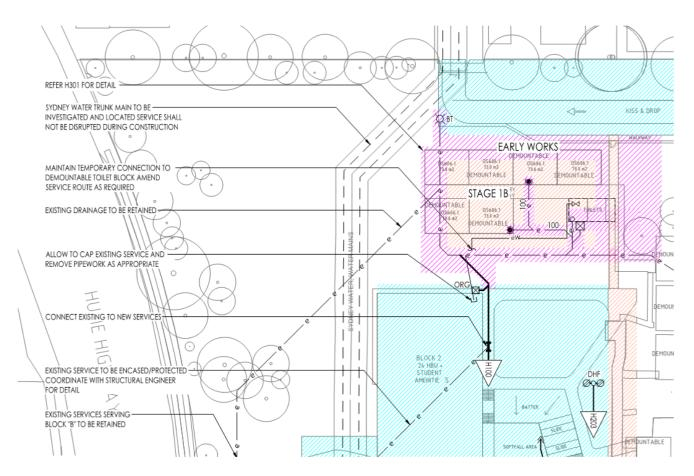
The primary sewer connection point is shown above serving the new building. The connection of existing waste water services to existing buildings shall be retained/diverted during construction to suit the orientation of the new building as required with any pipework that is damaged or unsuitable for retention to be replaced or relined using the specified pipe or relining material.
