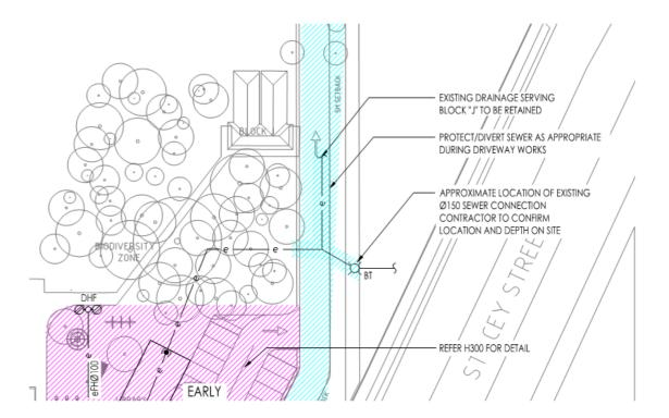
Secondary waste water connection shown above, serving existing block N, I and J shall be retained. The temporary library shall be connected to the existing waste water service as part of the early works phase.
