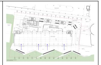
The Hall on level 1 will have access via lifts, stairs and escalators. There are multiple double leaf outward opening entry doors to Entry Terraces of the Hall on Level 1. The Hall on Level 1 leads to the terrace area which provides tiered seating viewing areas.
