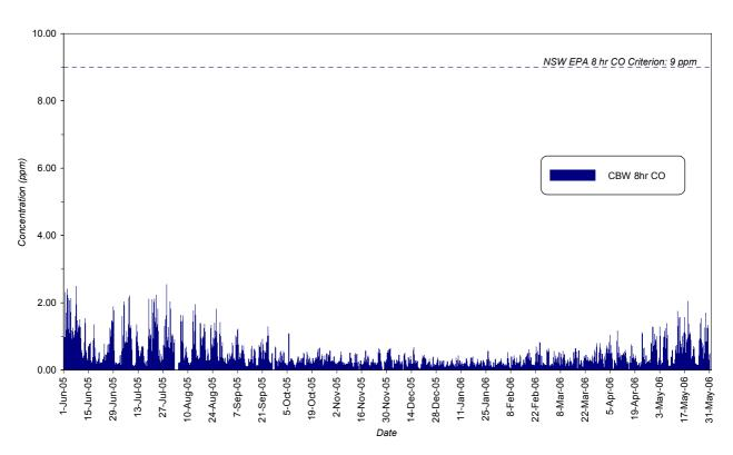
Figure 3.14: 8-Hour Rolling Average CO - CBW Monitor
