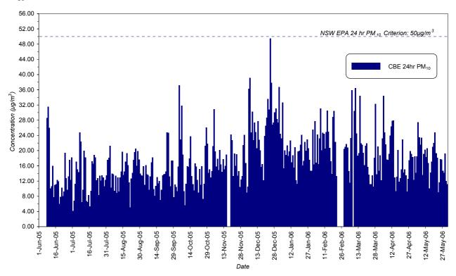
Figure 3.15: 24-Hour Average PM<sub>10</sub> – CBE Monitor
