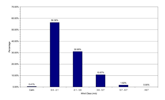
Figure 3.1: Histogram of Wind Speeds at CBE monitoring station, June 2005 – May 2006. Average wind speed is 2.16 m/s.
