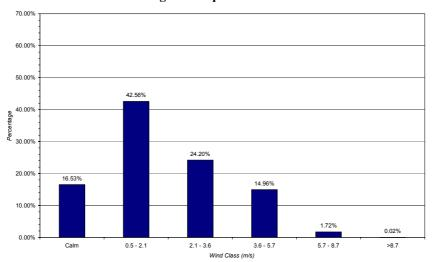
Figure 3.4: Histogram of Wind Speeds at NSW EPA Rozelle Monitoring Station', December 2000 – November 2001. Average wind speed is 1.96 m/s.
