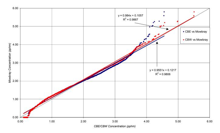
Figure 3.23: Ranked Scatterplot - CBE and CBW Vs. 'Project Station' - NO<sub>2</sub>
