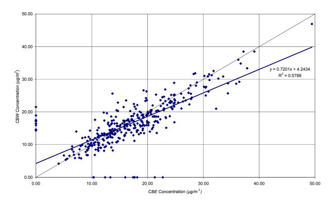
Figure A3: Scatterplot of Concurrent Observations - CBE Vs. CBW – PM<sub>10</sub>
