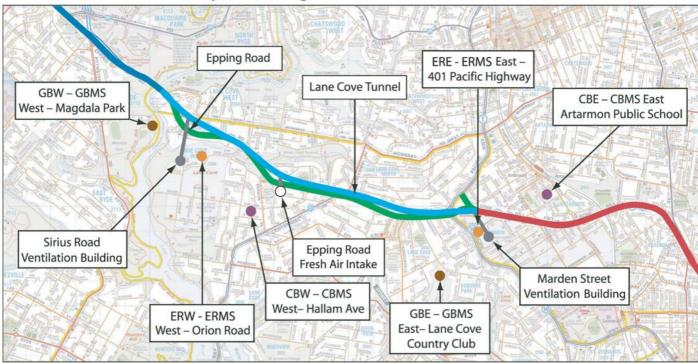
Figure 1.1: Lane Cove Tunnel Air Quality Monitoring Network
