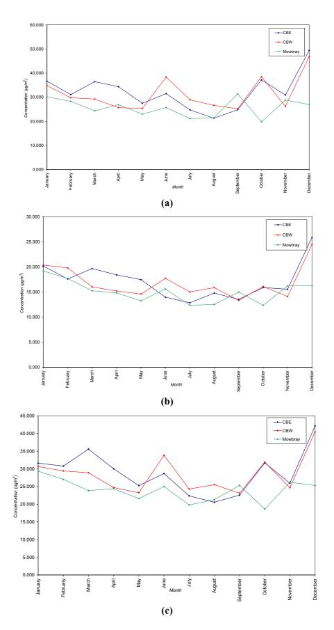
Figure 3.28: Time Series of Monthly–(a) Maximum, (b) Mean, and (c) Mean of Top 10%– PM<sub>10</sub>
