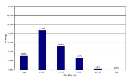
Figure 3.5: Histogram of Wind Speeds at NSW EPA Rozelle Monitoring Station, June 2005 – May 2006. Average wind speed is 1.92 m/s.
