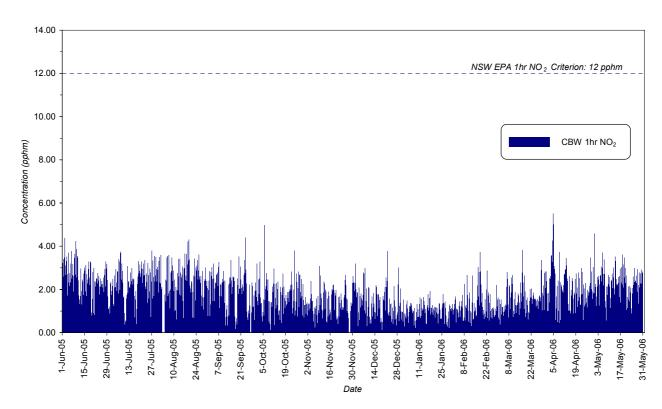
Figure 3.12: 1-Hour Average NO<sub>2</sub> – CBW Monitor
