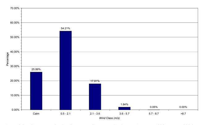
Figure 3.2: Histogram of Wind Speeds at CBW monitoring station, June 2005 – May 2006. Average wind speed is 1.19 m/s.
