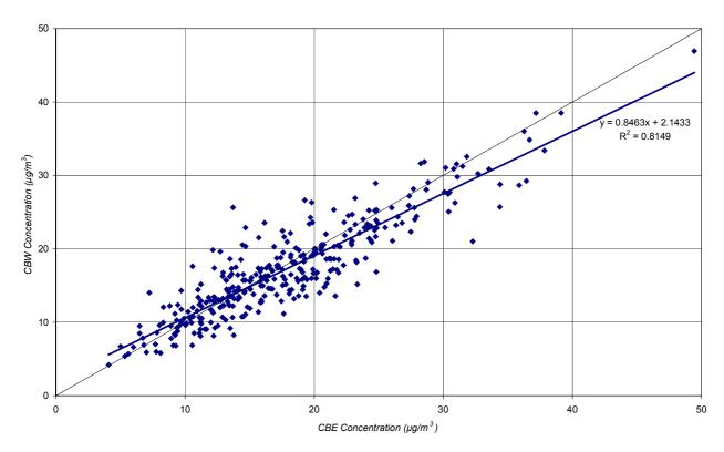
Figure A4: Scatterplot of Concurrent Observations - CBE Vs.  $CBW - PM_{10} - Zero$  values removed
