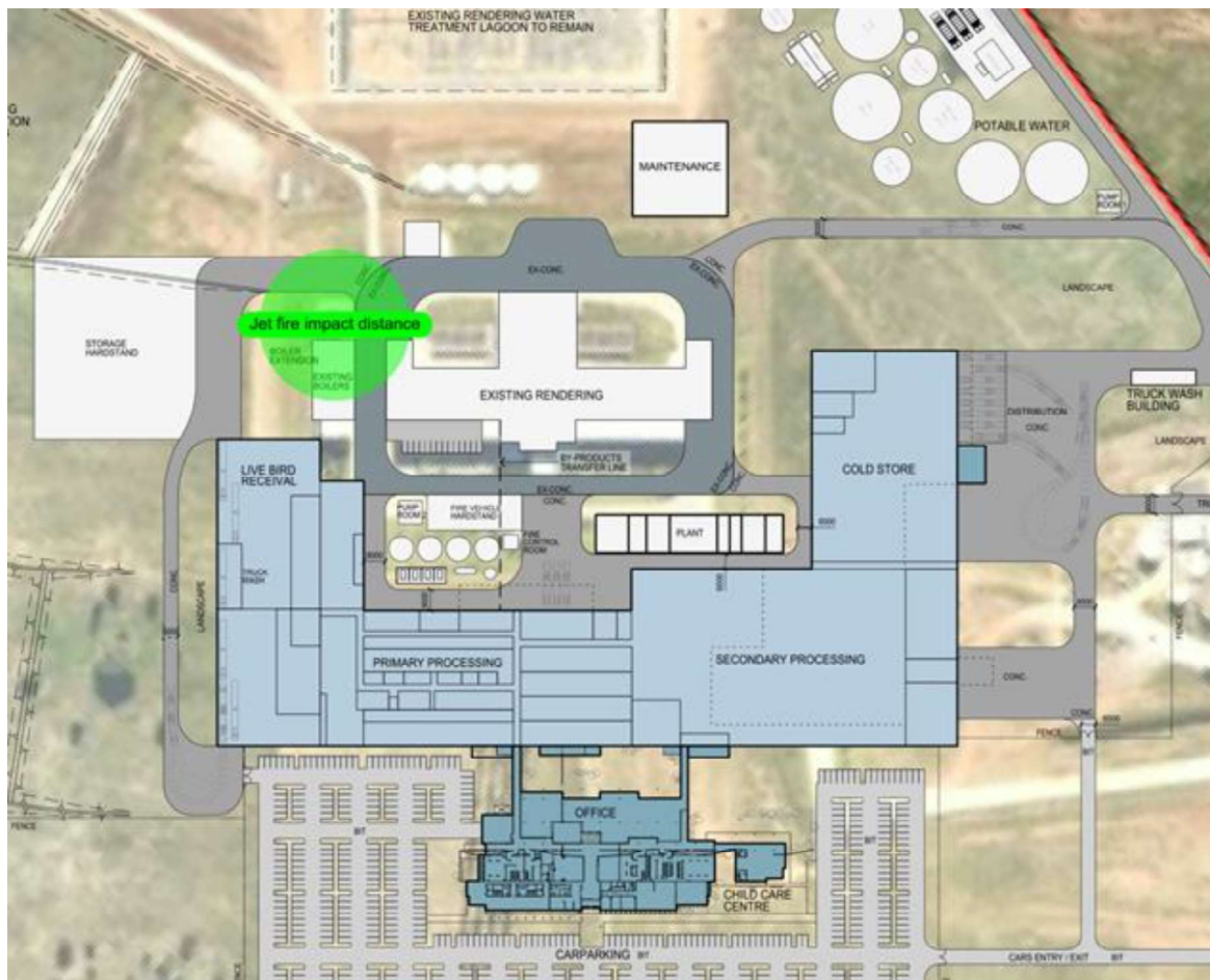
Figure 5-1: Impact from a Jet Fire
