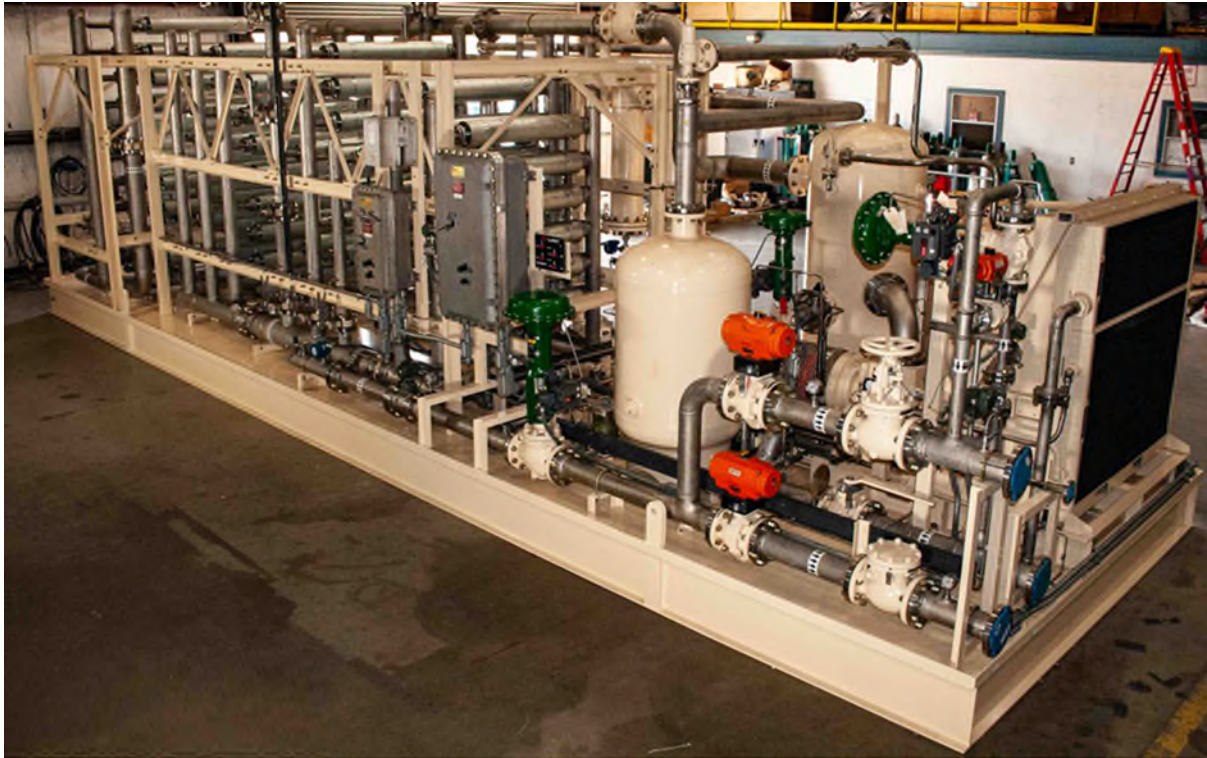
Figure 2.12 - Two Stage Gas Separation Module (Courtesy WGR/Generon)
