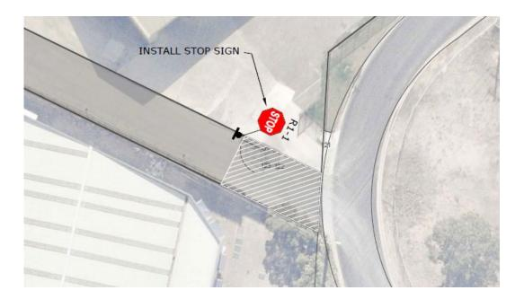
In the event that there are two vehicles travelling in the opposite direction, this would allow the drivers of both vehicles time to observe each other before entering the conflict area. At the site access driveway, there is adequate driver visibility between entering and exiting vehicles as shown below.
