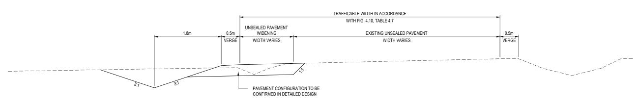
$\frac{\text{WIDENING LOCATIONS 2, 3 AND 4 - TYPICAL CROSS SECTION}}{\text{SCALE 1:50}}$
