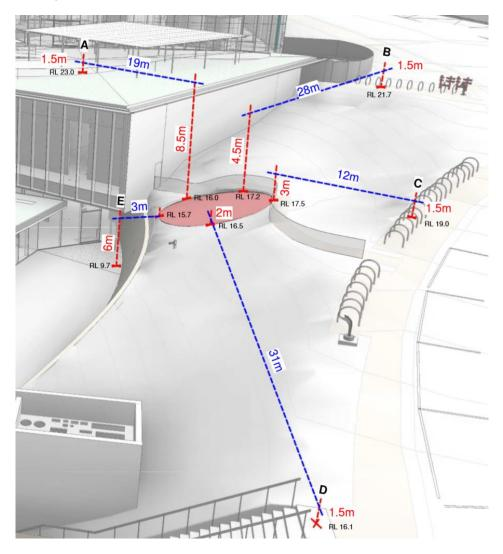
Points A through to D are all sufficiently far enough away in the horizontal plane to ensure there will be no perceived sensation from the cooling tower discharge. Point E is only 3m in the horizontal plane but sufficiently far below in elevation to ensure the discharge will not be physically perceived as the warmer air will be rising.
