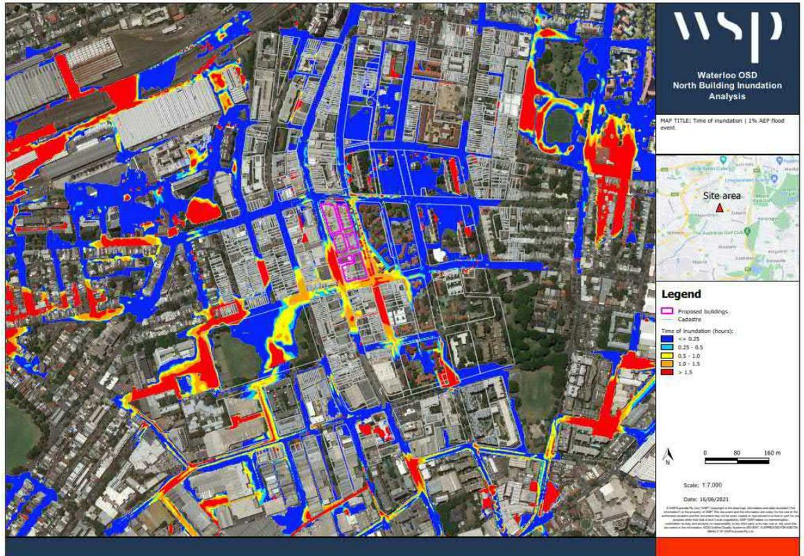
Figure 9: Time of inundation for the 1% AEP (25,60, 90- and 120-minutes storms) flood event
