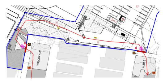
The primary access routes will be stabilised with crushed rock, a rumble grid and suitable sediment controls so to minimise off-site tracking of materials. Each gate will be equipped with a rock-check and wheel-wash station to further improve our impacts on the external road network.
