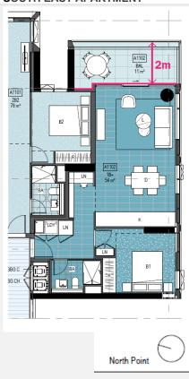
The living room glazing and balustrade line of the south eastern apartments is moved east by 240mm.
