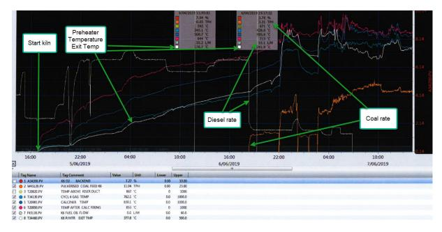
As can be seen on the above graph the kiln is starting up cold at approximately 17:00 on 5/06/2019. As previously described the diesel fuel oil is used to heat up the kiln and the preheater strings with the preheater exit temperature progressively increasing.
