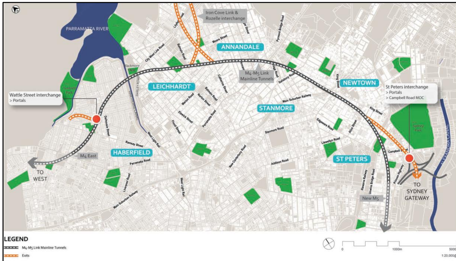
Figure 1 - M4-M5 Link Tunnel Overview
