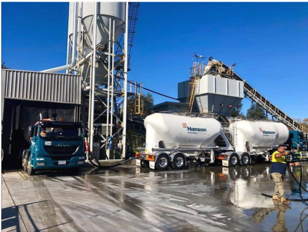
Plate 2 Photo of Cementitious Material Tanker Unloading at a Hanson Concrete Production Facility
