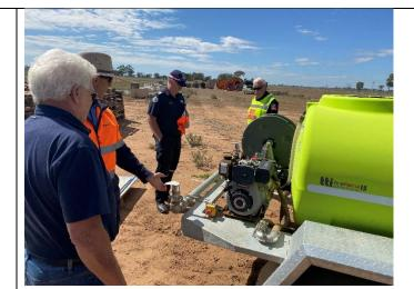
Inspecting on-site fire fighting equipment and valve compatibility with fire service equipment. This portable water truck is situated next to the main entrance point, site office and warehouse. Inspection tags are current and equipment well maintained.
