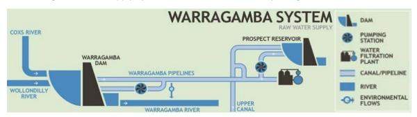
Figure 3-1 Warragamba Water Supply System (Source: WaterNSW)
