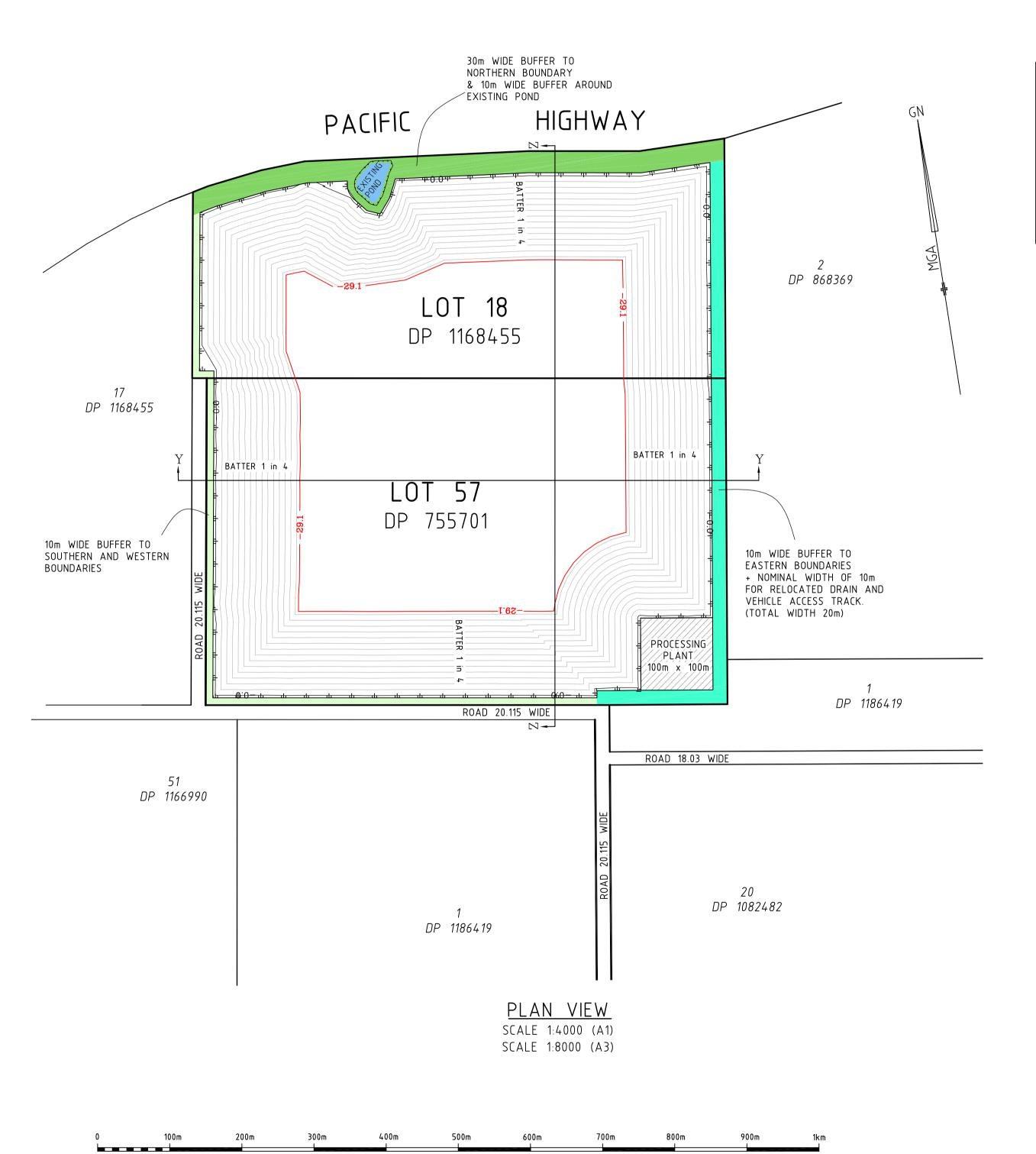
VOLUME COMPUTATION:EXCAVATE TO RL (AHD)VOLUME OF MATERIALRL -29.1 (DEPTH 30m APPROX)10,089,405 m³
