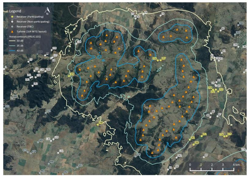
Figure 3: Mount Hope cluster - highest predicted noise level contours (corresponding to hub-height wind speeds of 9 m/s or greater)
