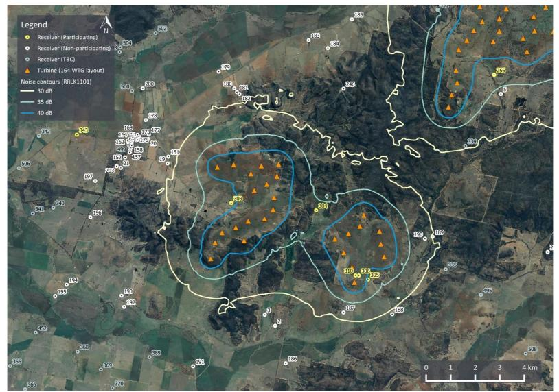
Figure 5: Leadville cluster - highest predicted noise level contours (corresponding to hub-height wind speeds of 9 m/s or greater)
