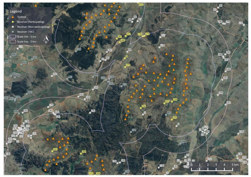
Figure 8: Proposed turbine locations and sensitive receiver locations – Black Stump cluster
