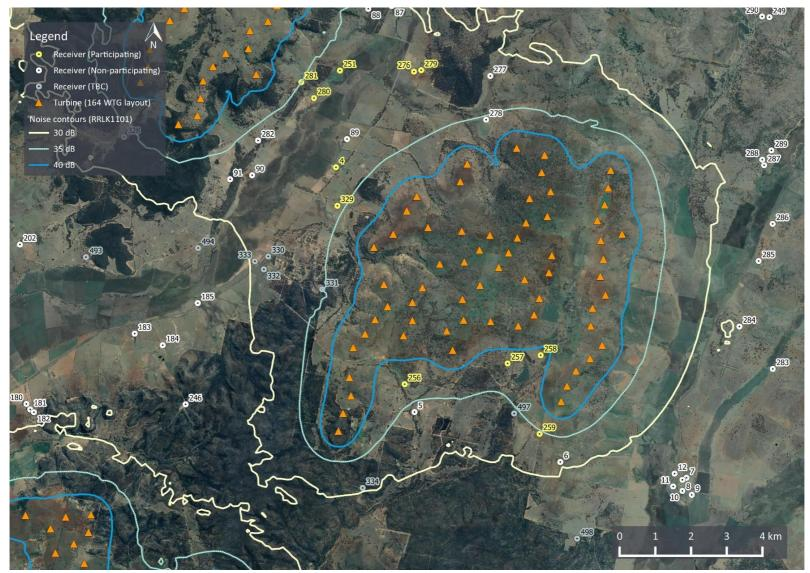
Figure 4: Black Stump cluster - highest predicted noise level contours (corresponding to hub-height wind speeds of 9 m/s or greater)
