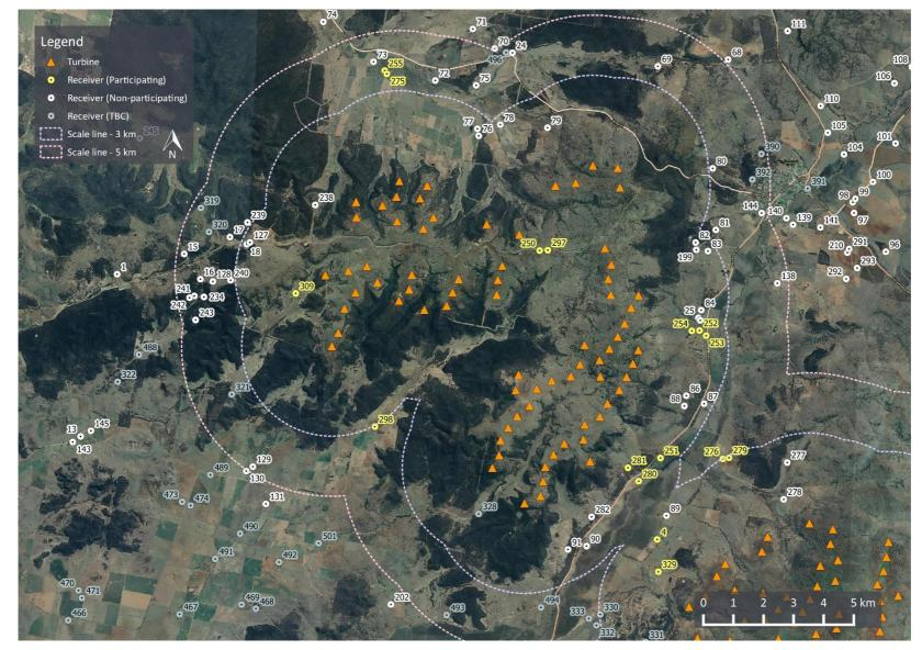
Figure 7: Proposed turbine locations and sensitive receiver locations – Mount Hope cluster
