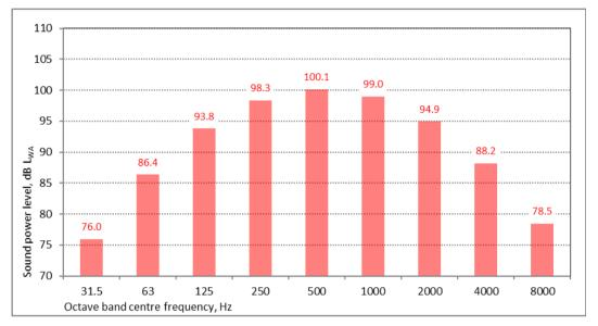
Figure 2: V162-5.6MW assessment sound power level spectrum, dB LwA
