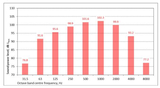
Figure 11: V112-3.0MW assessment sound power levels, dB L<sub>WA</sub>
