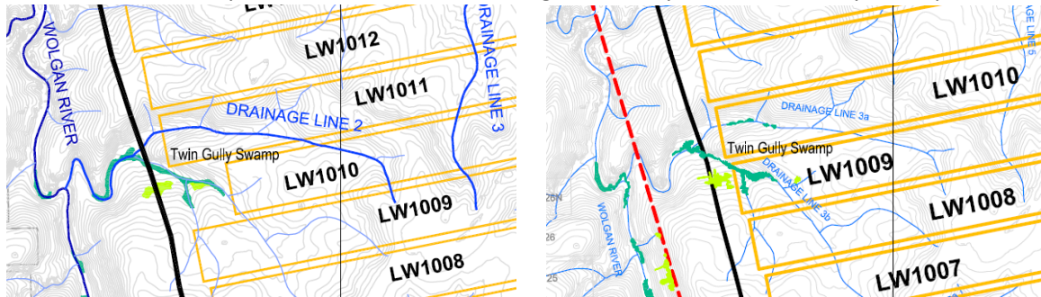
Longwall layout near Twin Gully Swamp in the 2014 (left) proposal and 2019 (right) proposal. Source: MSEC (2014, 2019)
