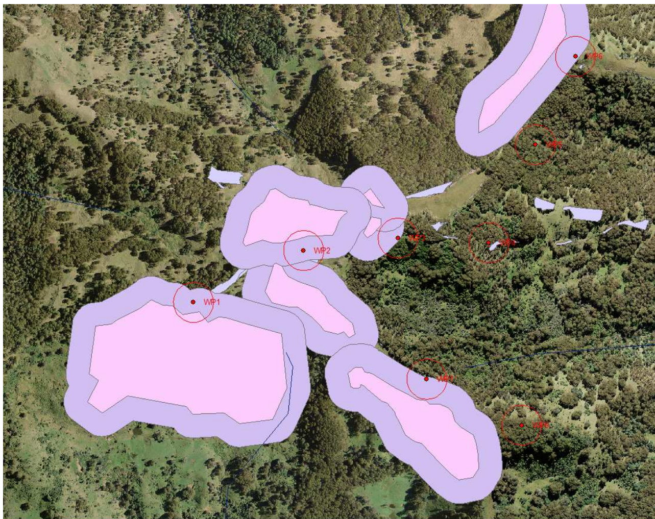
Figure 2: Location of turbines (red dots) in relation to cave bat roost polygons (pink polygons) and 100 metre buffers (purple polygons). Red circles are approximate blade swept area.
