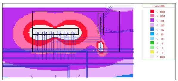
Figure 3.6a: Predicted magnetic field contribution associated with No 4 11kV riser - Carpark Level 4 (RL 9.5)
