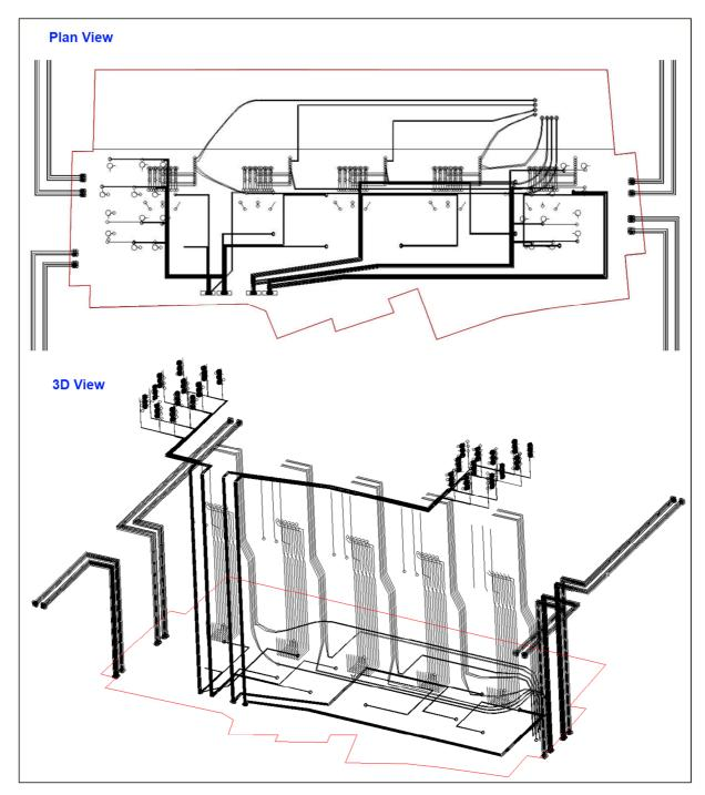
Figure 3.4 – CDEGS Model of proposed substation
