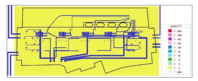
Figure 3.12: Predicted magnetic field contribution associated with the proposed substation – lowest level of commercial building (RL65.9)
