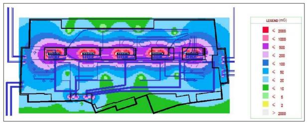
Figure 3.5: Predicted magnetic field contribution associated with the proposed substation - Carpark Level 3 (RL 6.35)
