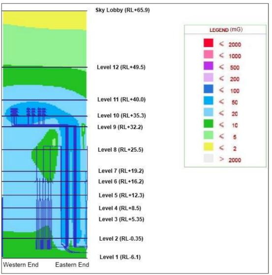
Figure 3.14: Predicted magnetic field contribution associated with the proposed substation -Southern wall, section A (the approx 1/3 of the wall towards the western end)
