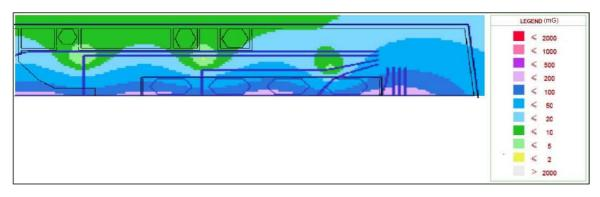
Figure 3.8: Predicted magnetic field contribution associated with the proposed substation - Commercial Building Management Office (RL 17.2)
