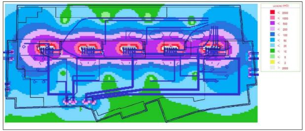
Figure 3.6: Predicted magnetic field contribution associated with the proposed substation - Carpark Level 4 (RL 9.5)
