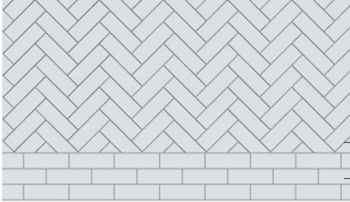
HERRINGBONE FACADE DETAILING
