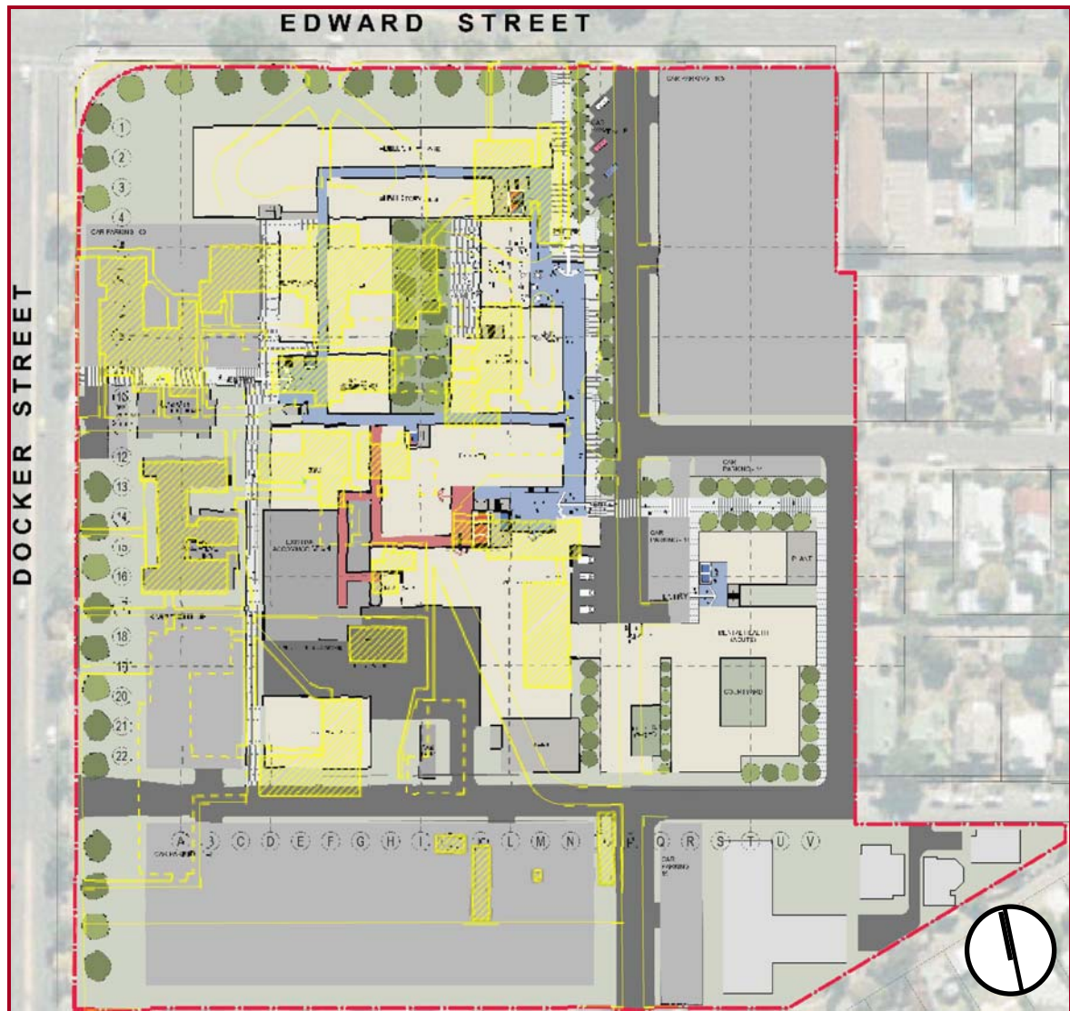
Figure 11: Overlay of the 1956 Wagga Wagga Base Hospital (yellow) over proposed development plan.
